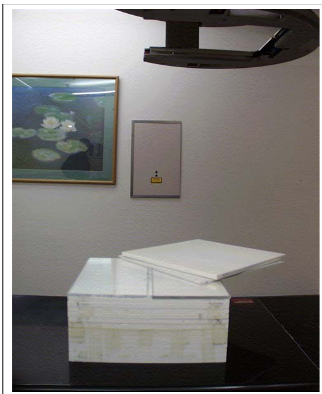
Figure 15. 3. TLD rods loaded into the stick bar shape holder for the profile curve measurement in different build up depth in solid slab phantom.
