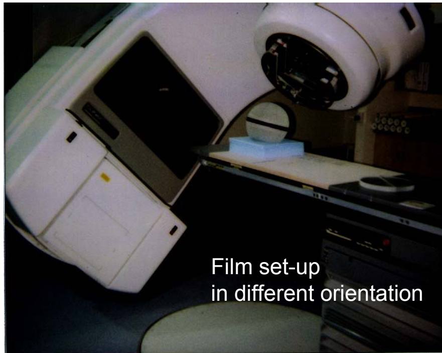
Figure 13.11 Ball phantom Film disk setup with different angle in three-D orientation.
