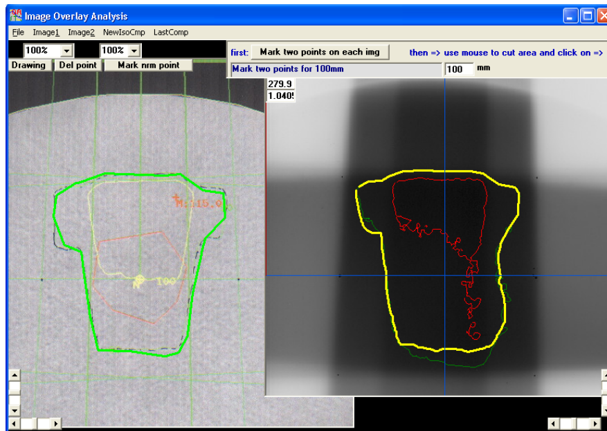
Figure 13.25 phantom lateral film dosimetry analysis result compare with planning calculation result
