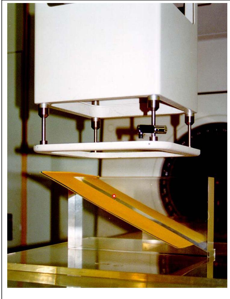
Figure 14.1 Film set up in solid wedge phantom used for Linear Accelerator electron energy check
