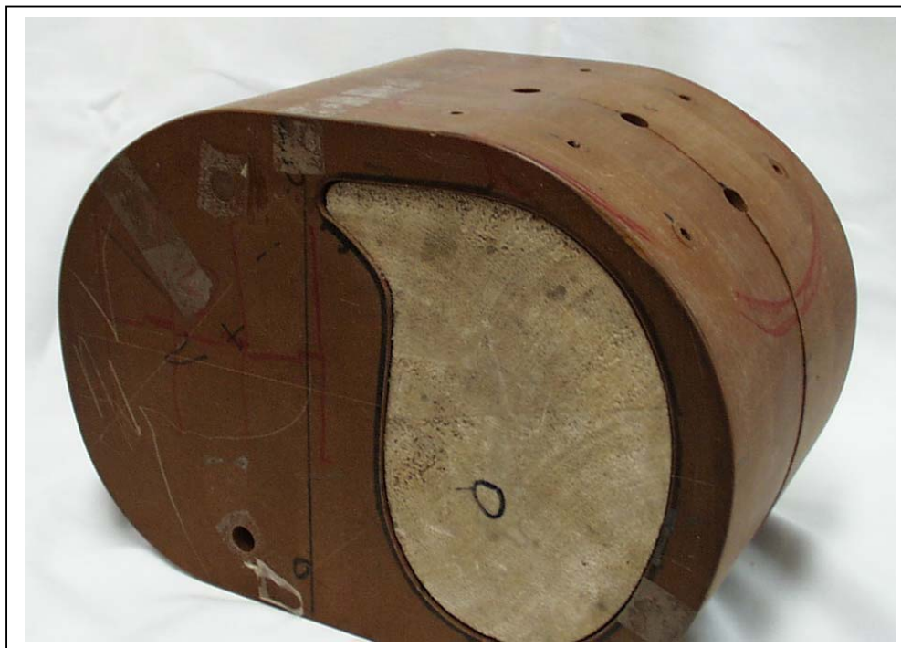
Figure 15.2. In-homogeneity solid water phantom used for chest wall point dose measurement using for TLD chips set up.
