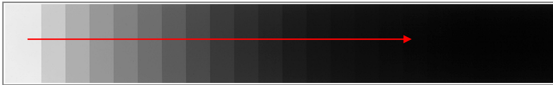
Figure 6.6 Kodak step wedge film bitmap image scanned by HP 4c/T desktop scanner and pixel value scan direction
