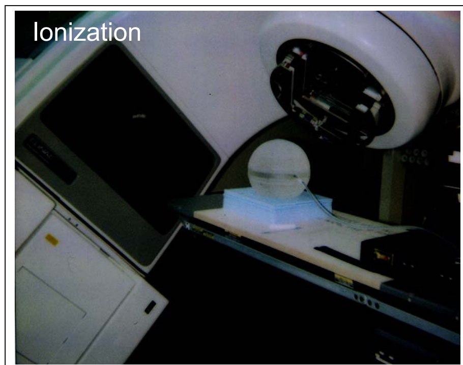
Figure 13.9 Ball phantom ionization measurement set up.
