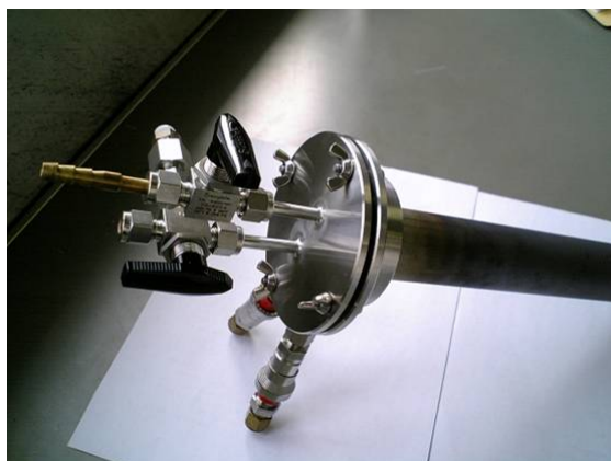
Figure 10.1: An image of the sealed tube furnace, which allow no contact with air over the whole procedure in this work.
