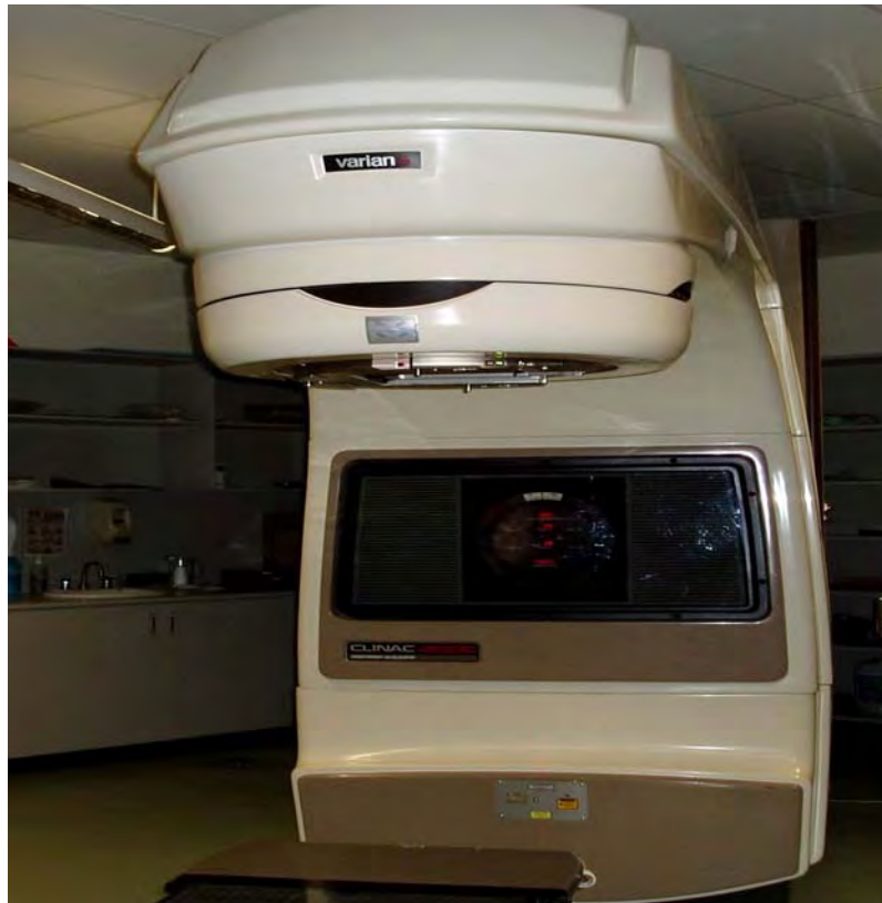
Figure 3.2. Picture of Varian Clinac 2100C linear accelerator. This machine is capable of producing 6 and 18 MV x-ray beams and 6, 9, 12, 16, and 20 MeV electron beams.
