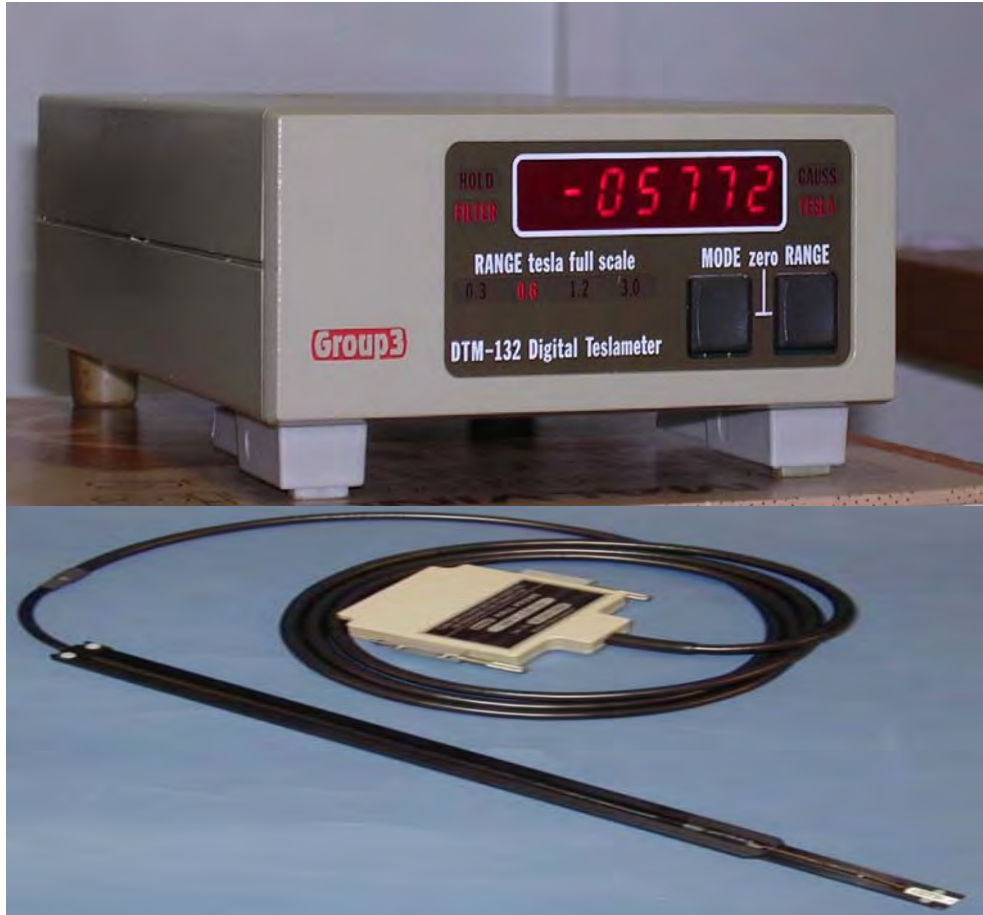
Figure 3.17. Pictures of the DTM-132 Digital Teslameter and Hall probe.
