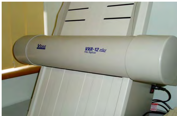
Figure 3.14. Picture of Vidar VXR-12 Plus film digitiser for scanning film.
