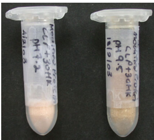
Figure 3.1 Photograph of the CLP modified with 3OHKyn at pH 7.2 on the left; and CLP modified with 3OHKyn at pH 9.5 on the right. CLP was incubated with 3OHKyn at 37°C for 48 hours. As can be seen the protein modified at pH 7.2 was pink and the protein modified at pH 9.5 was brown.
