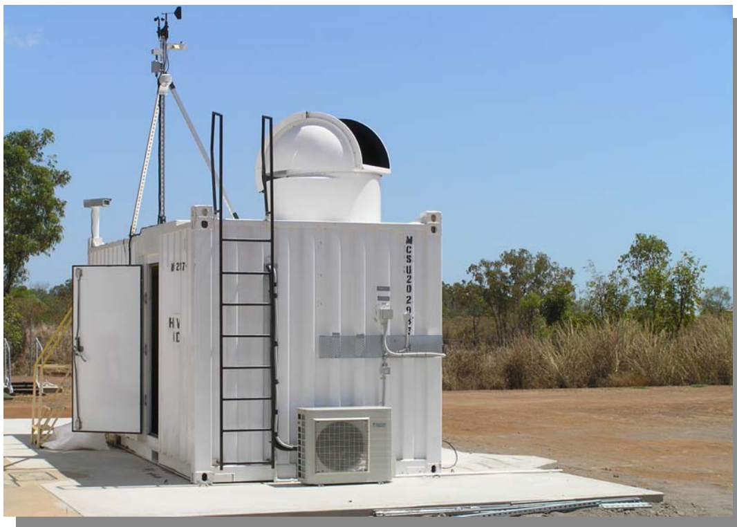
Figure 5-1: Photograph of the TCCON observatory at Darwin showing the container, tracker dome and weather station.
