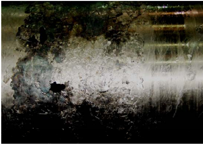
Figure 7.9 Strip welding (roll B in Figure 7.7)
