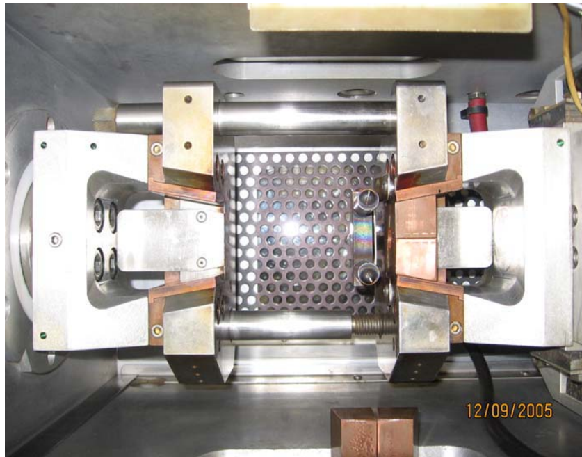
Figure 2.6 Gleeble system chamber (elevated view)
