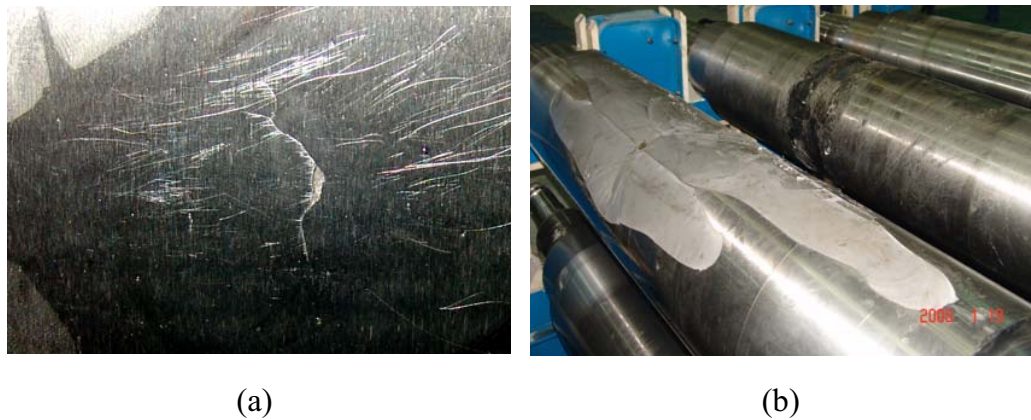
Figure 7.2 Spalling of work rolls: (a) roll D and (b) roll A.
