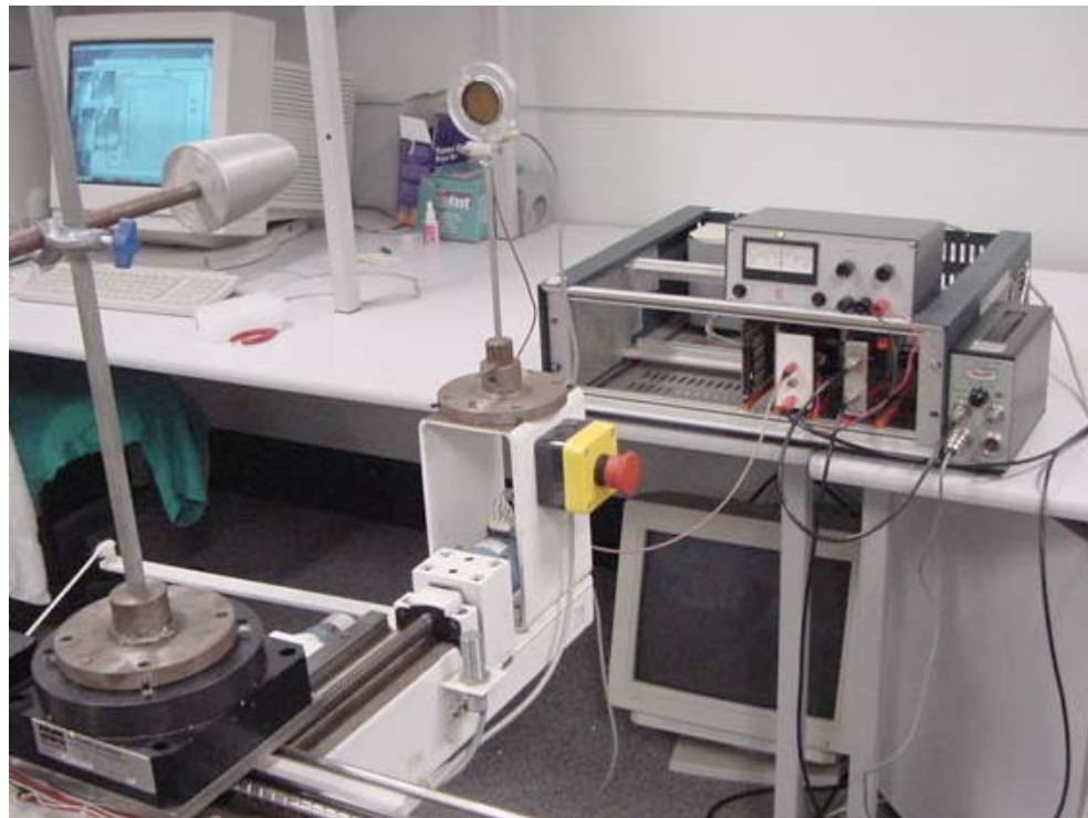
FIG. 4.1. Experimental set-up used for chirp transmission and echo reception.
