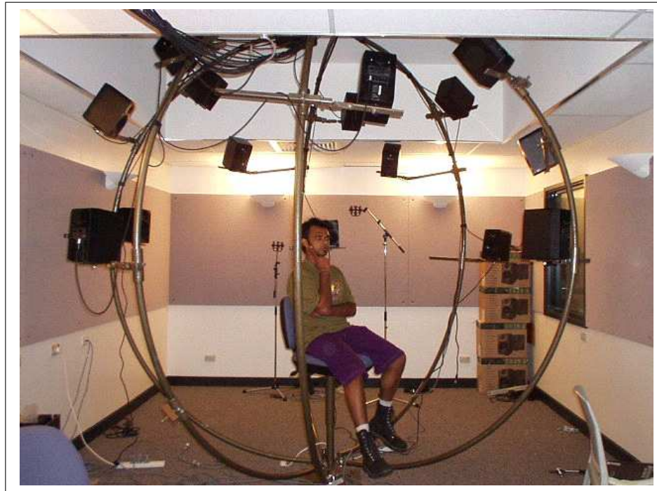
Figure 5.2: The configurable speaker array of the CHESS system
