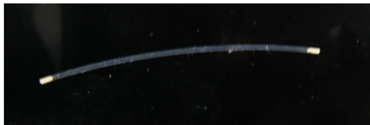
Figure 5.7: The capillaries filled with FDG used inside the tubes of the phantom
