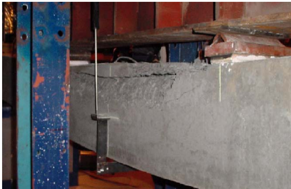
Figure 5.10 Steel U shape from base side to support LVDT for measuring midspan deflection.
