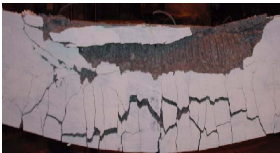
Figure 5.14 Cracking at ultimate load for beam R12P25-A105
