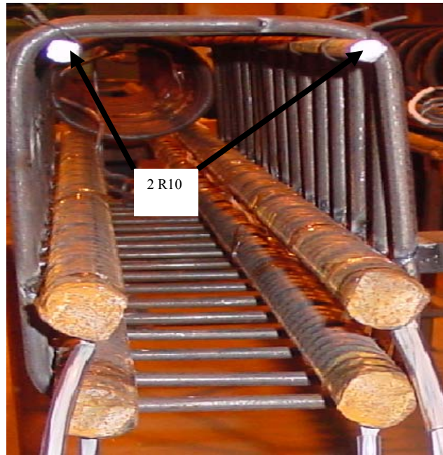
Figure 5.5 Beam Cage cross section
