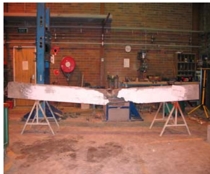
Final deflection of Beam N8P75-A80
