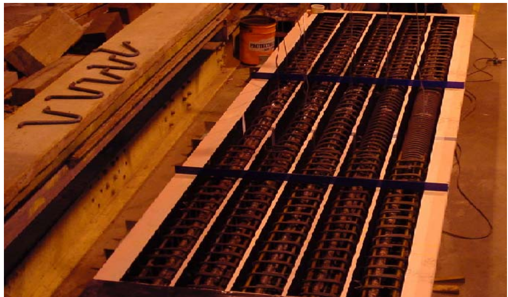
Figure 5.2 Five beams with different helical pitch in wooden formwork
