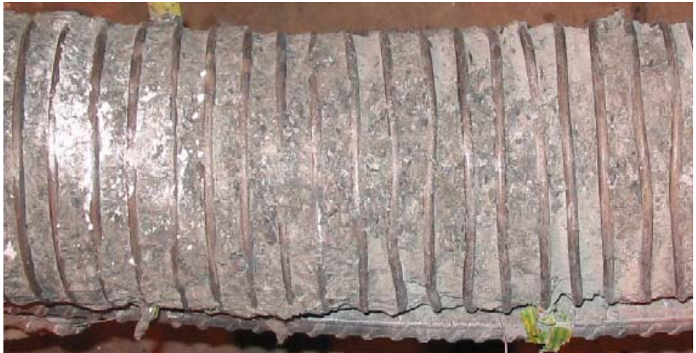
Figure 6.11 Core concrete of Beam 8HP25
