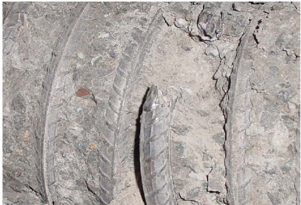
Figure 6.26 The rupture of the helical confinement of Beam N12P35-D85 at welding point.
