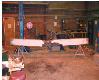
Final deflection of Beam N8P100-A80
