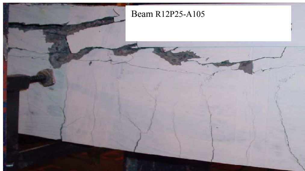
Figure 5.13 Cracks just after spalling off concrete cover
