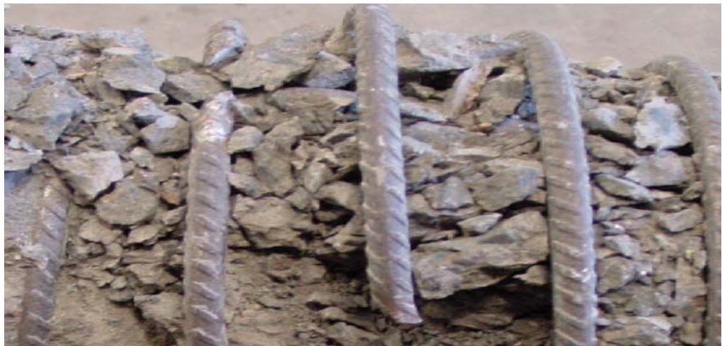
Figure 6.29 Disintegration of the confined core of Beam R8P35-D85
