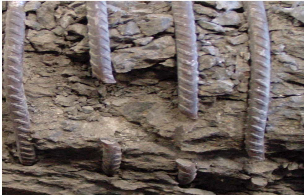
Figure 6.28 The rupture of the helical confinement of Beam R8P35-D85
