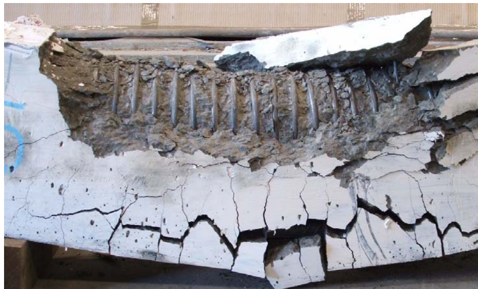
Figure 6.21 Crack patterns for Beam R10P35-C95
