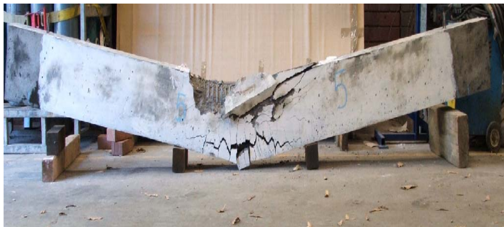
Figure 6.19 Ultimate deflection of Beam R10P35-D95
