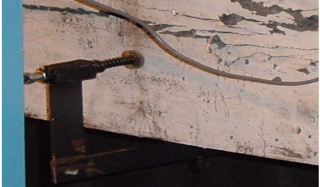
Figure 5.11 Steel U shape from rapper side to support LVDT to measure midspan deflection
