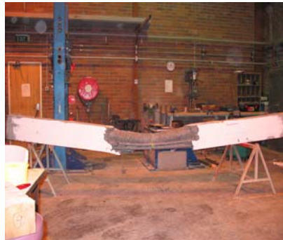
Final deflection of Beam N8P25-A80
