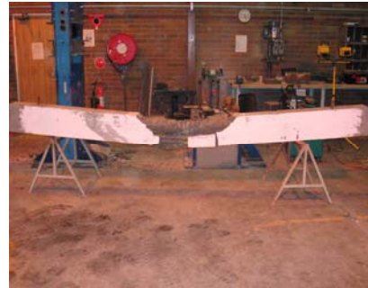
Final deflection of Beam N8P50-A80
