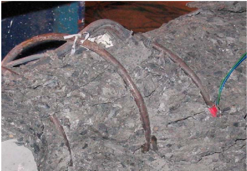
Figure 6.12 Buckling in the steel bar of Beam 8HP100
