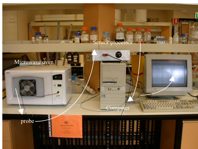
Figure 2.23: View of method of SAR calibration. Fluoroptic probes were inserted through the meshed door of the microwave oven and held in place in the cuvettes. The probes were connected to the sensor processor, which in turn was connected to a computer where the data was logged.
