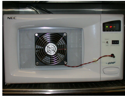
Figure 2.9: View of the remodelled oven during a pulse period (red light).
