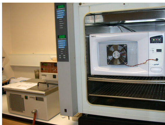
Figure 2.14: View of microwave oven placed inside the incubator (door open). The circulating water-bath (on left) was connected with two water hoses that entered through the back panel of the incubator (not visible), then through two holes of the back panel of the microwave oven and the infusion bags inside the oven (see also Figure 2.13).
