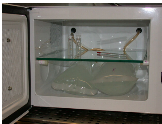
Figure 2.13: View of cavity of the microwave oven showing the two infusion bags filled with circulating water. The bags were inter-connected by a tube. The left bag is connected to the hose of the water-bath that pumps water out into the bags and the right bag is connected to the hose that delivers the water back to the water-bath. The hoses fit through holes in the back panel of the incubator. The two incubator doors (not shown on the photograph) were closed during the experiment.
