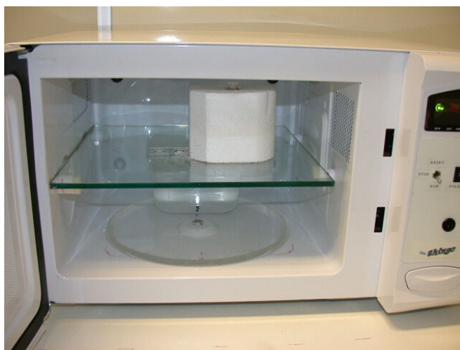
Figure 2.17: View of the opened microwave oven as described in the Exposure system 2 . The glass plate turns on a perplex clip. To avoid temperature loss, exposure was performed on the cuvette containing the protein solution while placed in a polystyrene box. The SAR was determined also with the cuvette placed in the box.
