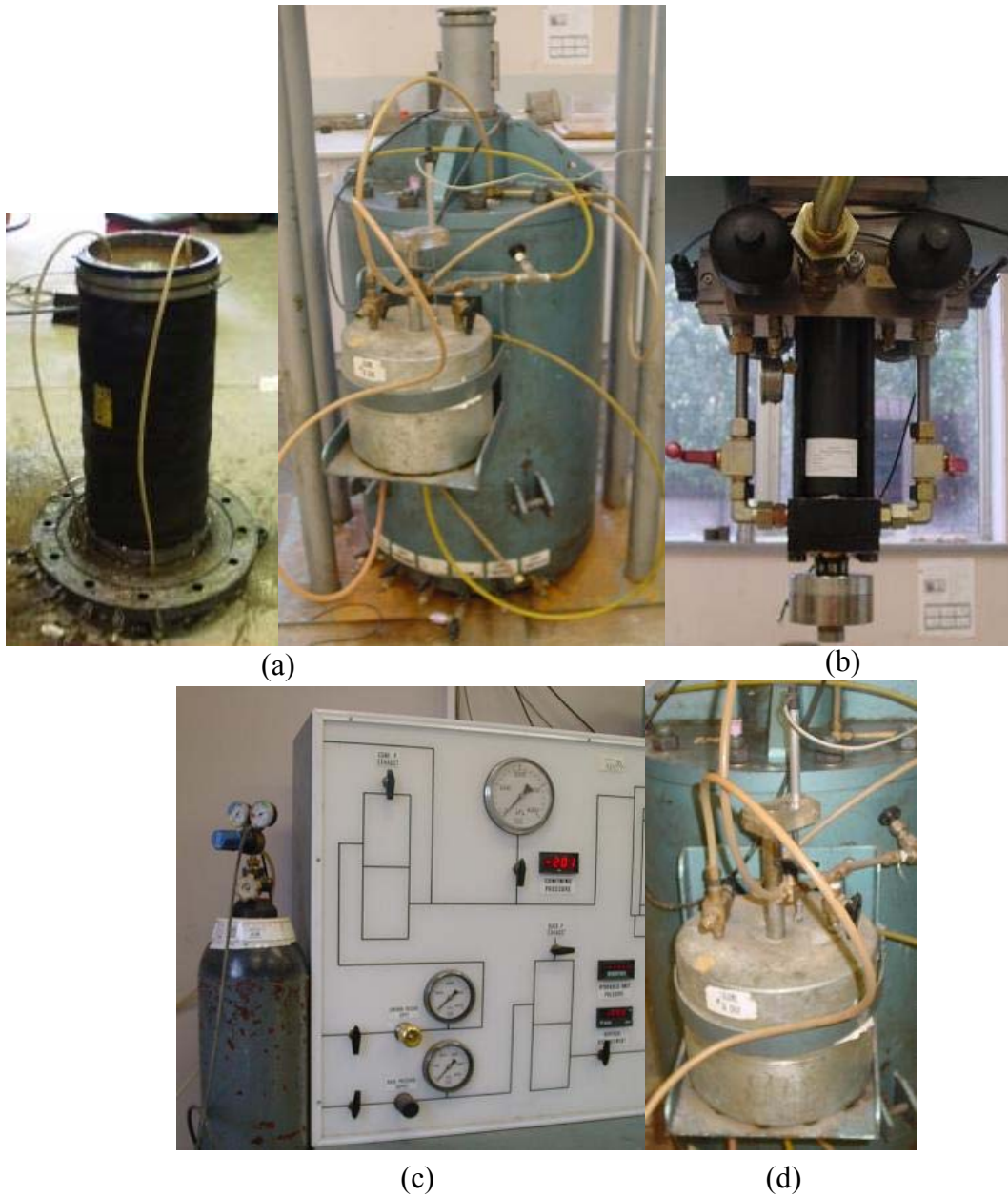
Figure 3.2 Additional details of the testing apparatus, (a) The triaxial chamber and membrane, (b) The dynamic actuator, (c) The confining pressure system, and (d) The volume change measurement device
