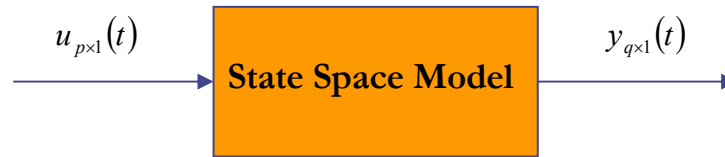
Figure B- 1 state space model relates ‘p’ inputs to ‘q’ outputs using ‘n’ first order ordinary differential equations.
