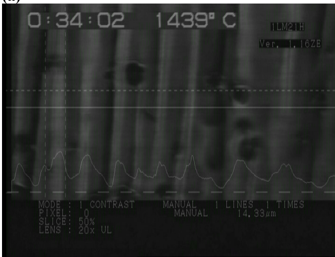
Figure 4.5a-b: (a) A sample of an image used to measure surface diffusion in \gamma & \delta -iron, \gamma - iron, T = 1300^\circ \text{C} . Here the scope trace measures a section of the topography of two grain boundary grooves. (b) This is an image of a sinusoidal pattern made by mechanically etching the surface \delta - iron, T = 1440^\circ \text{C} .
