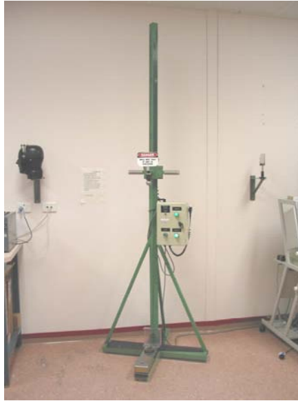
Figure 5.14. Standard drop ball test instrument.
