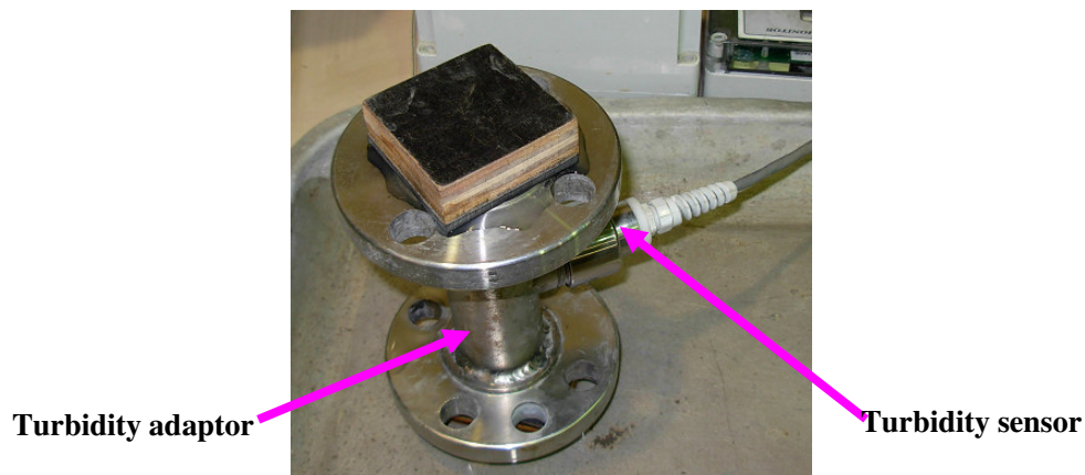
Figure 4.9 Arrangement to determine the relationship between turbidity and concentration
