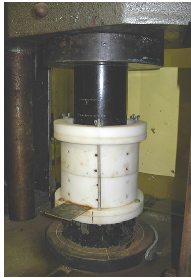
Figure 4.15(b) Compaction of soil with AVERY compression machine
