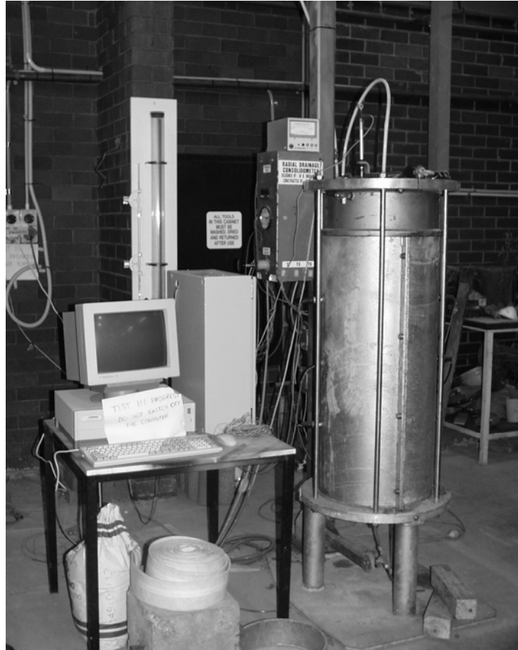
Figure 4.1 Large-scale consolidometer
