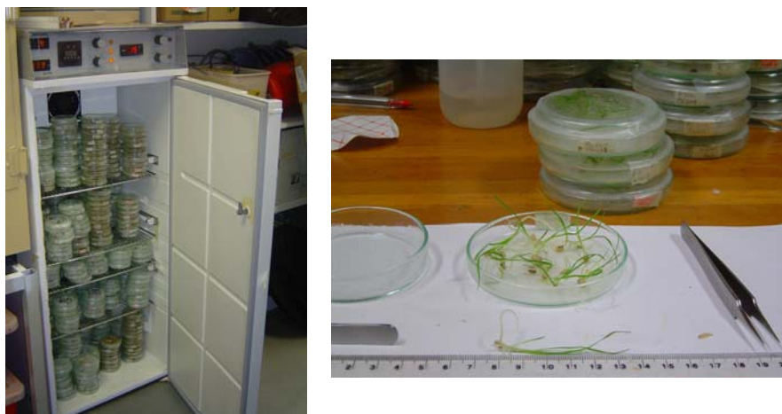
Figure 4.2: The bioassays were run in an incubator (left) and seedling shoot and root lengths were measured (right).
