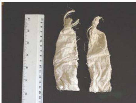
Figure 6.1: Photograph of calico, resin-filled bags.
