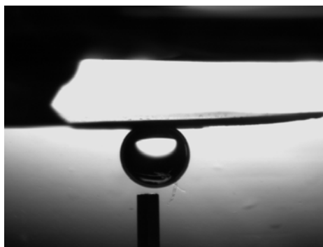
Figure 38. Electrochemical contact angle measurement of captive water bubble resting on the underside of PTTh.ClO 4 -coated Pt sheet. The potential was switched between +0.8 and 0 V vs. Ag/Ag + .
