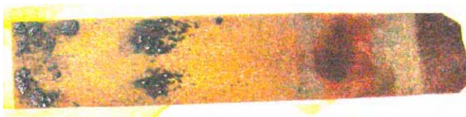
Figure 5.22- Potentiostatic deposition of polyaniline doped with ferrocene sulphonic acid onto aird Industries Ni-Cu-coated polyester at 750 mV over 1 hour.
