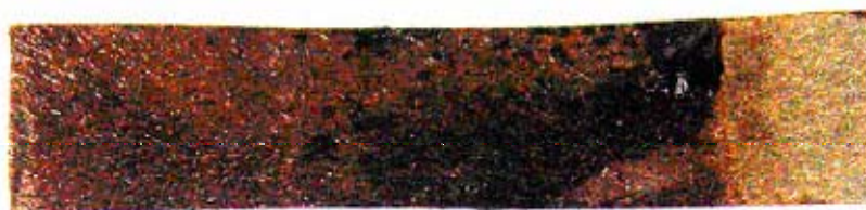
Figure 5.20- Galvanostatic deposition of polyaniline doped with ferrocene sulphonic acid onto Laird Industries Ni-Cu-coated polyester at 3 \mu\text{A}/\text{cm}^2 over 16 hours.
