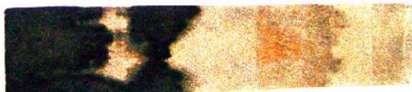
Figure 5.21- Galvanostatic deposition of polyaniline doped with ferrocene sulphonic acid onto aird Industries Ni-Cu-coated polyester at 3 \mu\text{A}/\text{cm}^2 over 2 hours.
