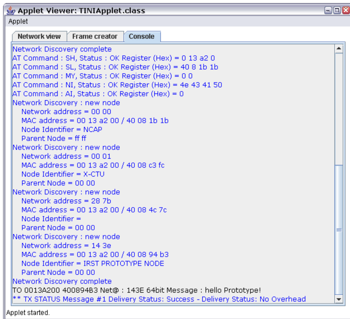
Figure A-3: View of the HMI's console. This displays and explains all the frames transiting through the bridging node
