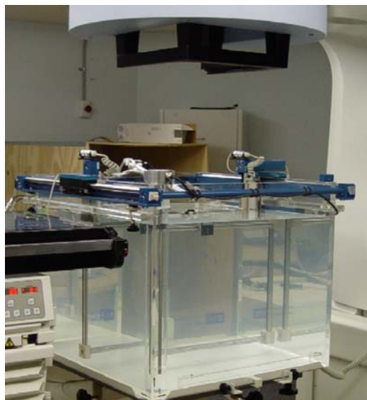
Figure 4.1 Wellhöfer water tank place under Siemens linac.
