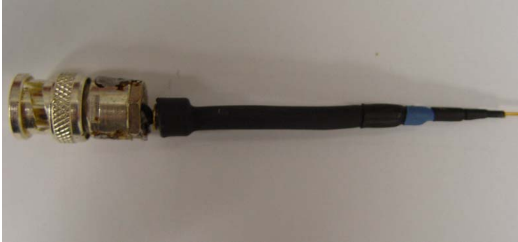
Figure 3.5 Picture of Design 1. Photodiode contacts were soldered on BNC triaxial connector.
