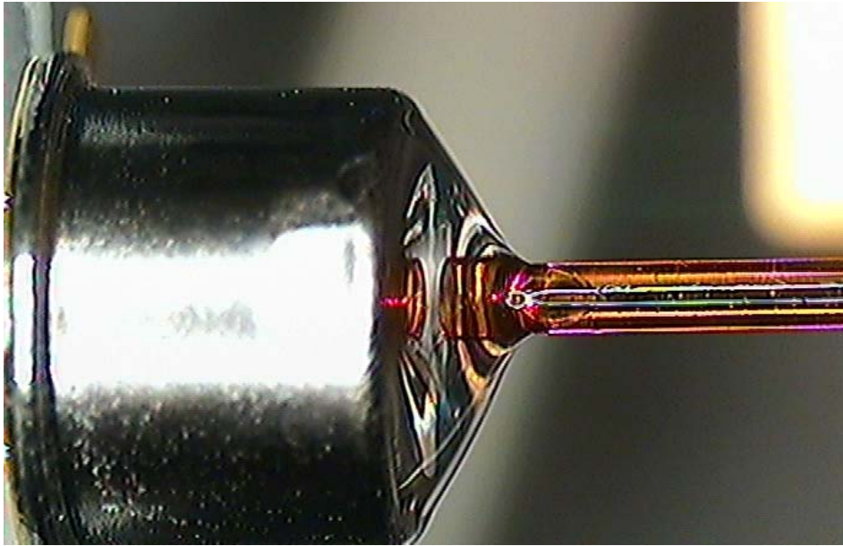
Figure 3.3 Silica Alignment of silica optical fibre on photodiode prior to ultraviolet curing. Epotek epoxy was poured between the silica optical fibre and the photodiode.
