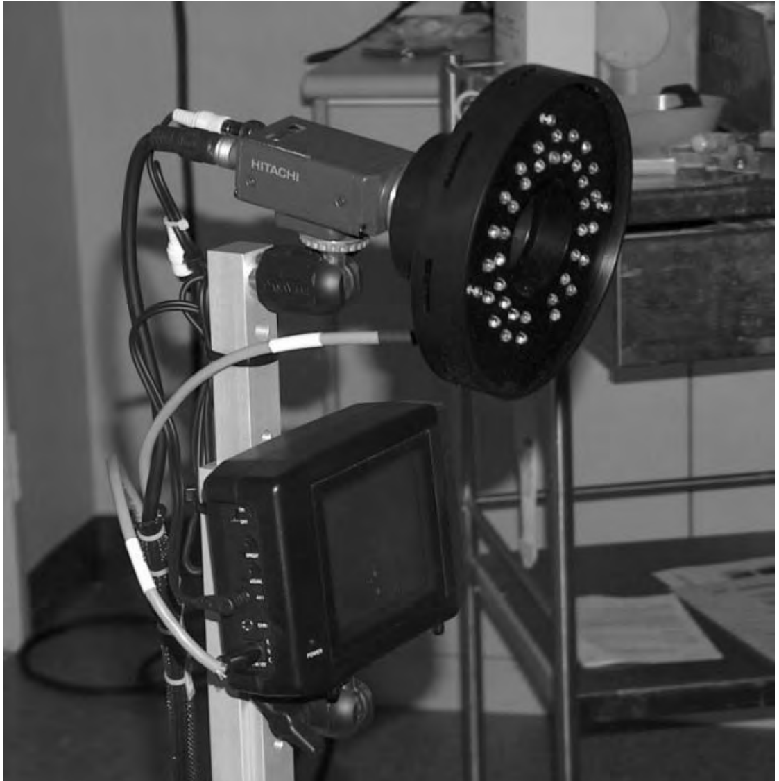
Figure 2.5: RPM CCD camera surrounded by infrared LEDs, and display monitor.
