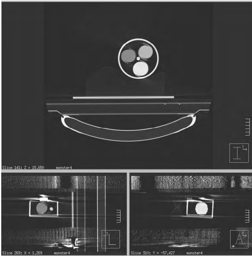
Figure 3.18: Pinnacle 3 user interface illustrating artifacts observed for 50% inspiration reconstruction, 2.4 cm amplitude movement, 10 respirations per minute (6 s period). Window 1601, level- 300.
