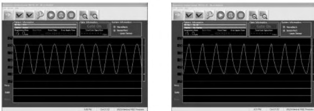
Figure 3.7: Two modes of movement offered by the Anzai Respiratory Gating Phantom; Normal (left) or Resp. (right).
