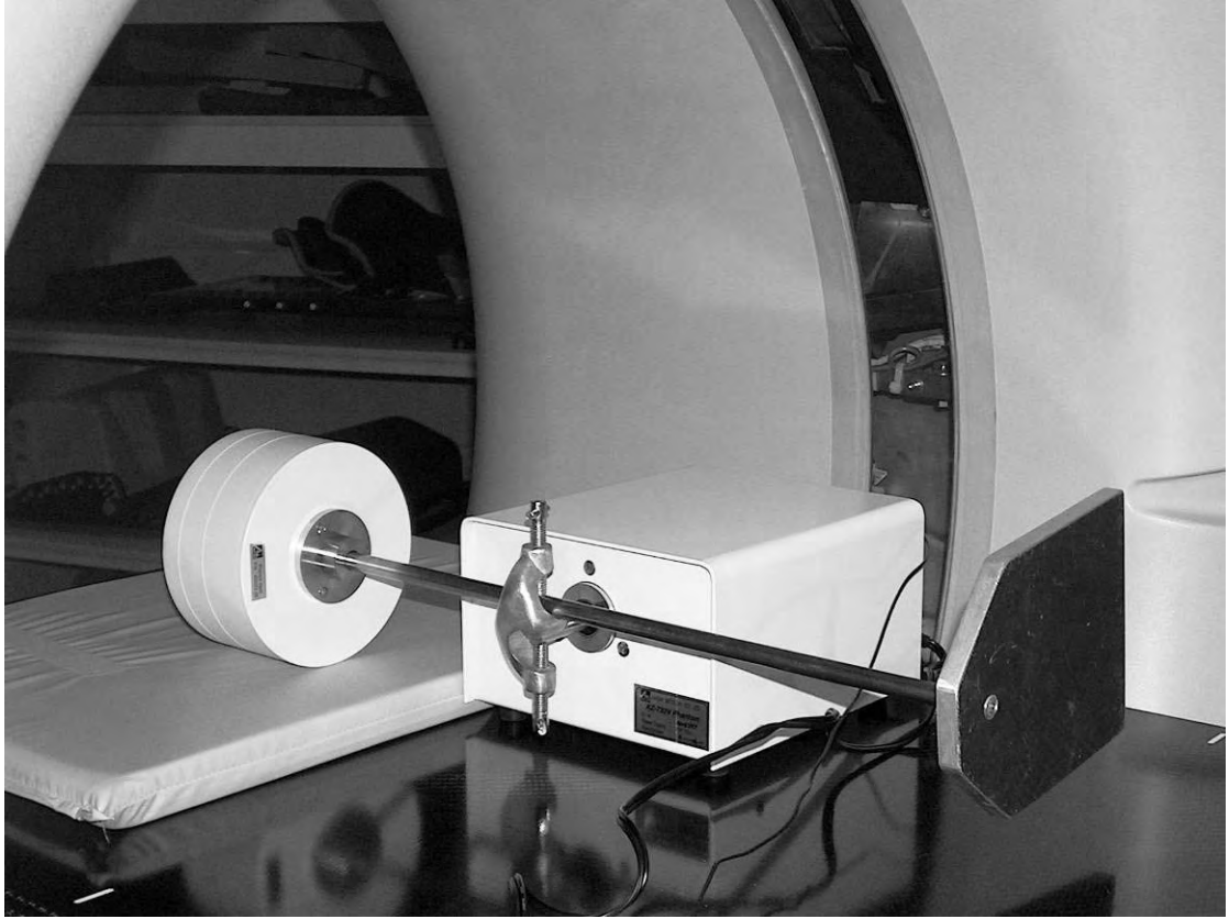
Figure 3.10: Experimental set-up for gated measurements with phantom movement in scan plane.
