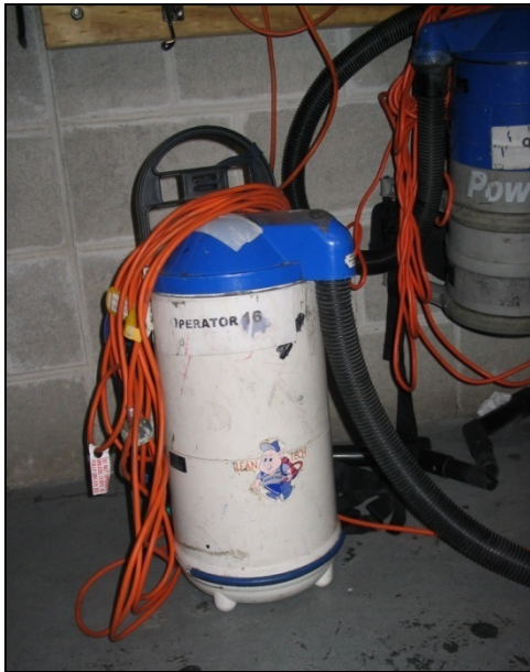
Figure 2.4: Examples of a back pack vacuum cleaning machine.
