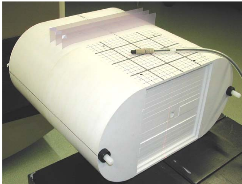
Figure 3-4. Scanditronix-Wellhöfer I'mRT phantom used for IMRT verification measurements, shown with the head and neck cube towards the front, with lateral scattering bodies in place, and the torso phantom at the rear. The phantom is also shown with a CC13 chamber and film inserted.
