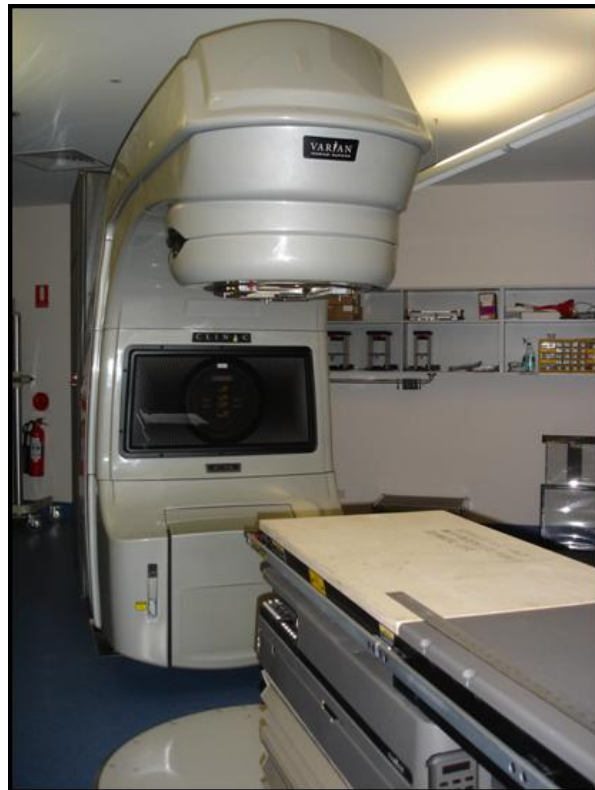
Figure 3-1. Varian 2100EX linear accelerator used for all measurements in this project. The linac is capable of producing both 6MV and 10MV photon beams (although only 6MV was used in this project), as well as multiple electron beam energies. It is equipped with the Varian Millennium TM MLC-120 multi-leaf collimator system.
