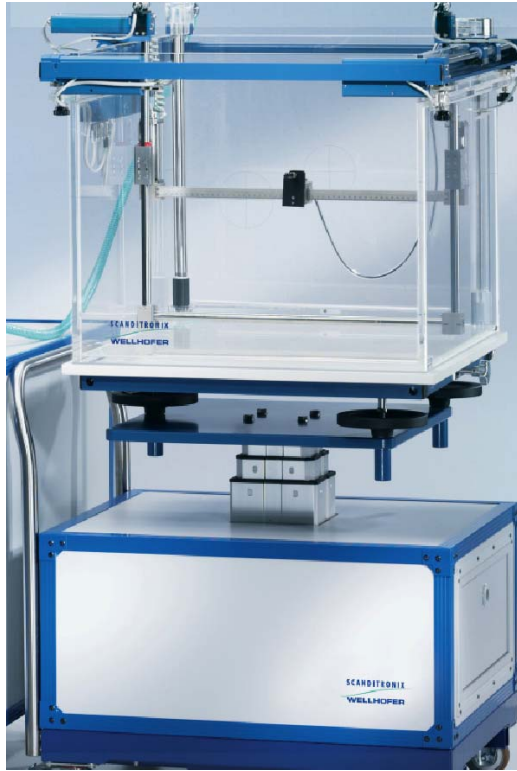
Figure 3-6. Scanditronix-Wellhöfer 3D water phantom (Blue Phantom) used to collect depth doses and beam profiles used in RadCalc calculations.
