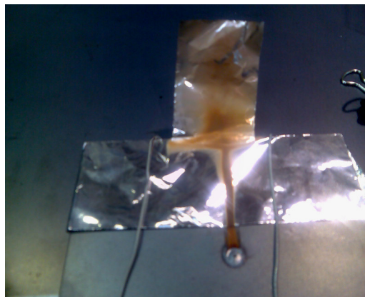
Figure 3-13: The Aluminium foil, holder bar and generated fume after removed from chamber.
