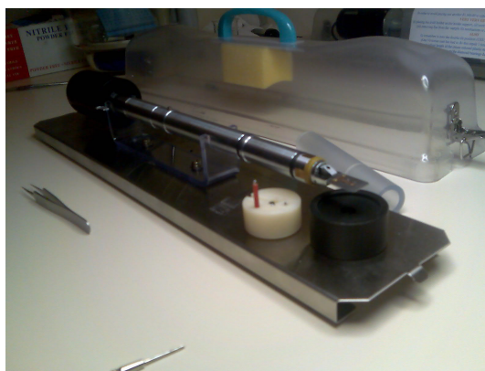
Figure 3-23: The specimen was placed in the single-tilt TEM grid holder.
