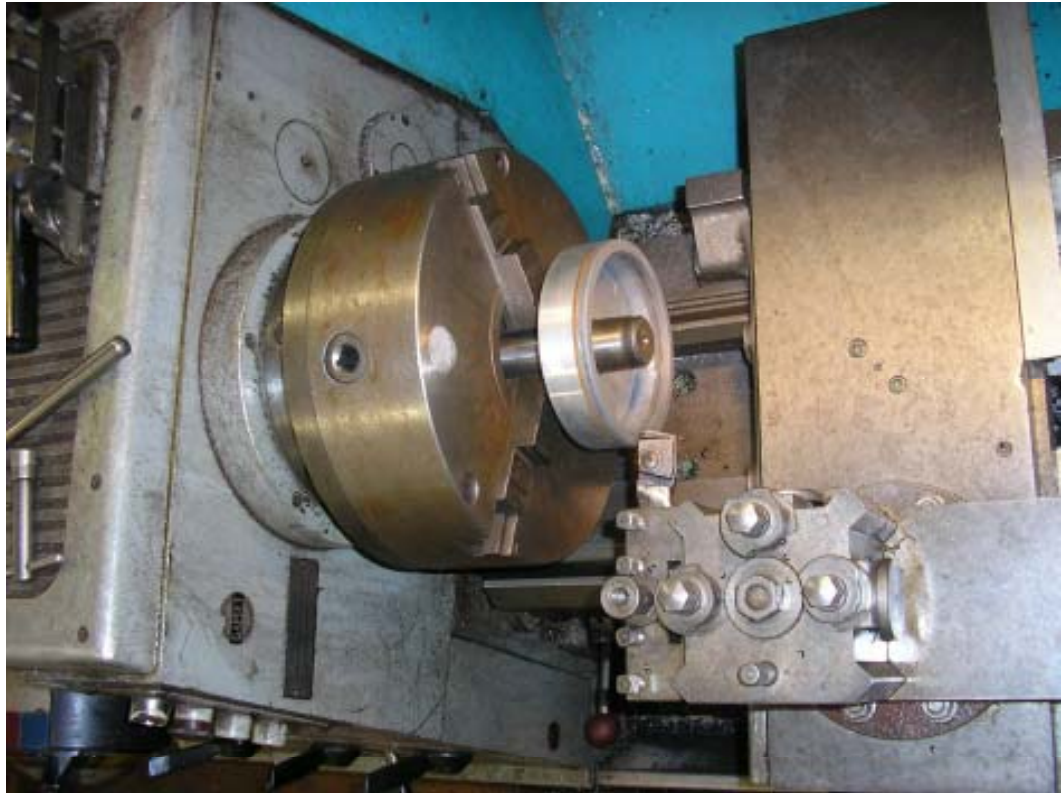
Figure 2.2.6 Top view of the second grinding machine setup
