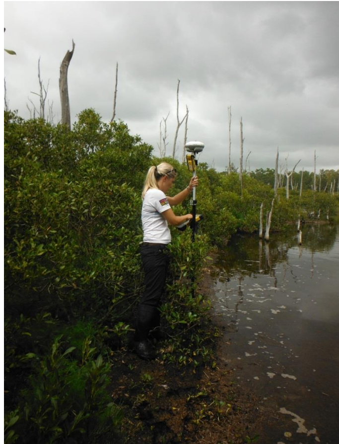
Figure 4-1 Real Time Kinematic (RTK) positioned to collect xyz data at Chain Valley Bay, Lake Macquarie for the purpose of obtaining geographic positions and elevations at core locations.
