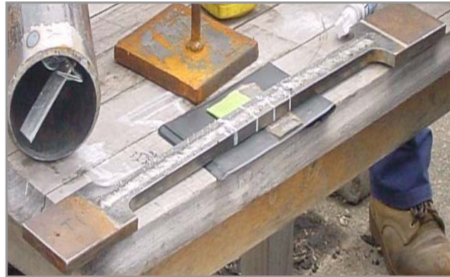
Figure 5.3 A 460mm long weld bead was deposited on a 660mm reduced tensile specimen. Here the specimen is being prepared for x-ray analysis.
