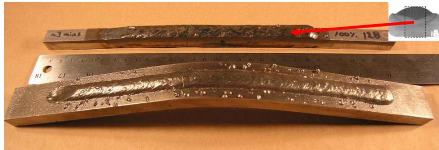
Figure 5.4 Single bead on plate arrangement for all bend specimens. The narrow specimen is at the top of the image and the dotted line (top right) represents the cross section of the narrow bend specimen.
