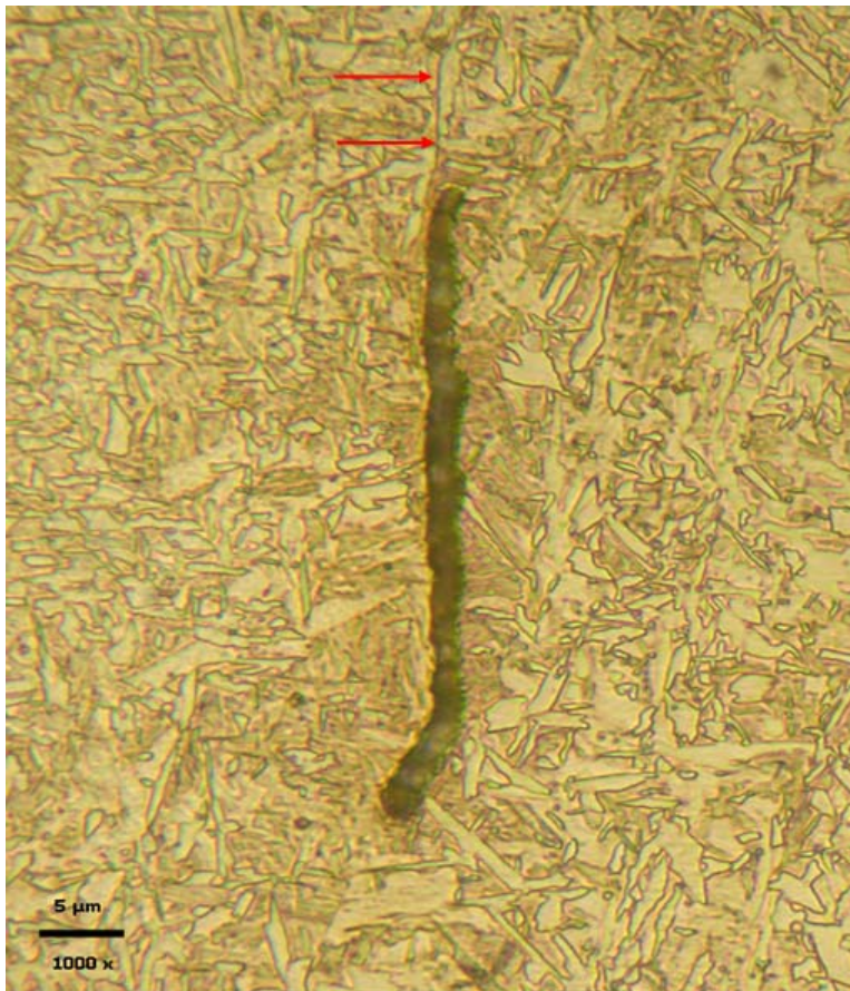
Figure 7.15 Image of a microcrack in a region sparse in PF(G). The faint black line arrowed at the top of the crack indicates a prior austenite grain boundary.
