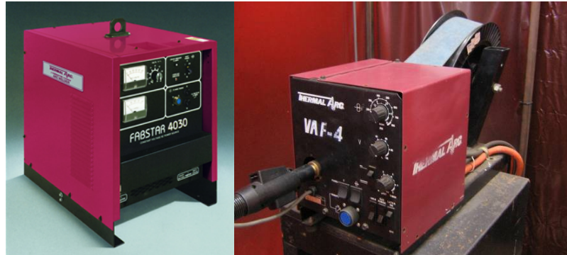
Figure 4.1 A constant voltage MIG power source (Fabstar 4030) together with an associated wire feed unit was used to produce the welds required for the tensile and bend test specimens.
