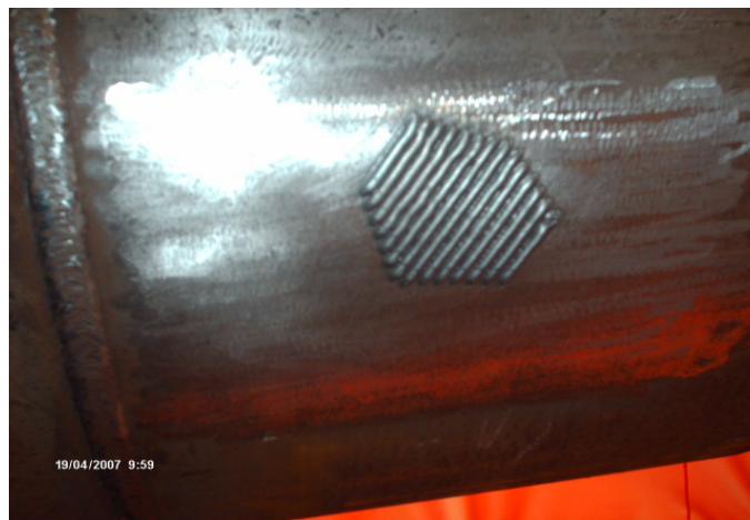
Figure 6.5-2. Weld trial 1 on pipe.
