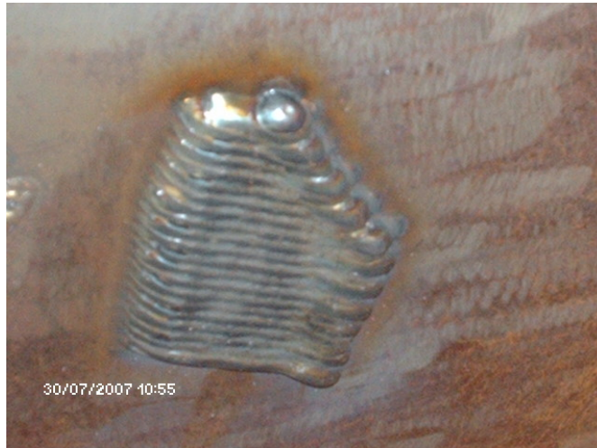
Figure 6.5-3. Weld trial 2 on pipe.
