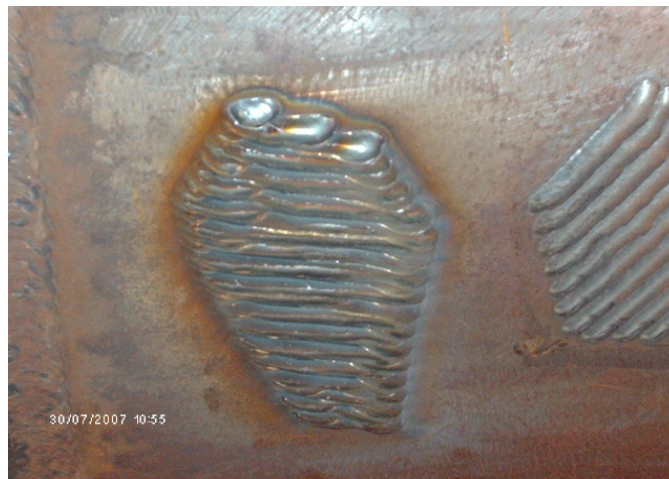
Figure 6.5-4. Weld trial 3 on pipe.
