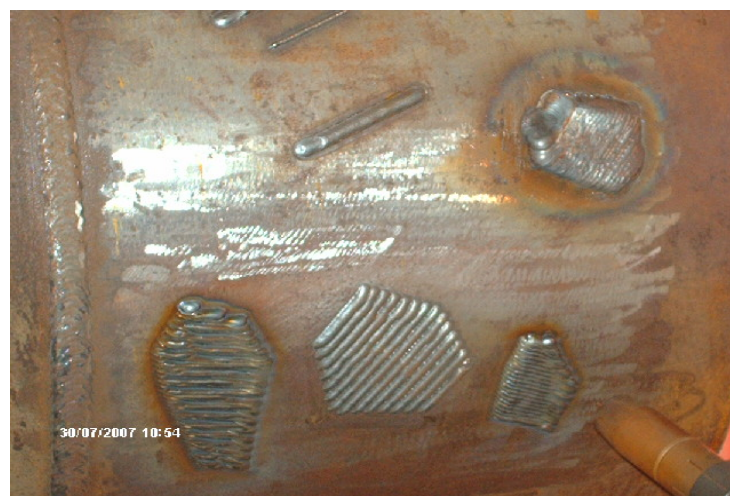
Figure 6.5-5. Various weld trials on pipe.
