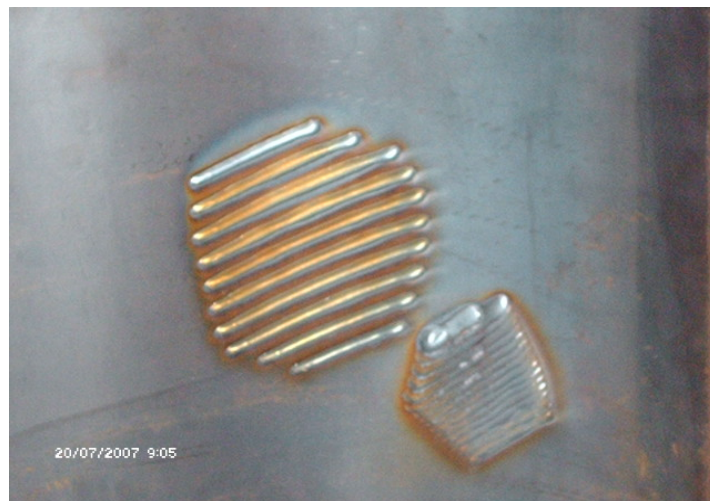
Figure 6.5-7. Weld trials on curved surface.
