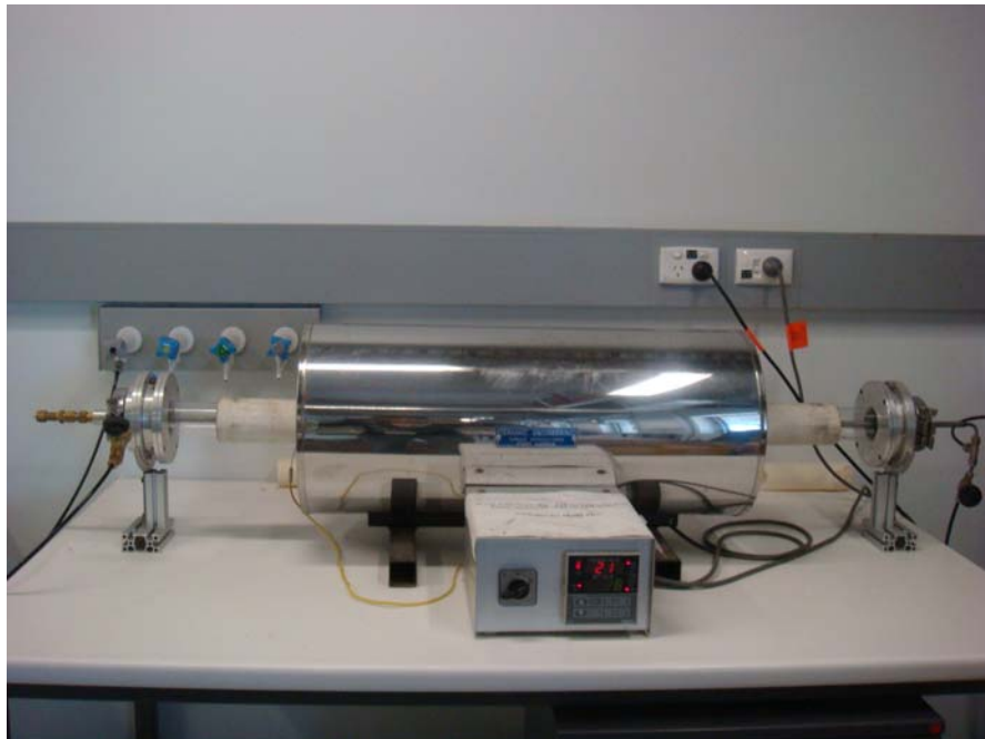
Figure 2.1 Horizontal tube furnace with gas end-caps includes vacuum system and controlled atmosphere apparatus.
