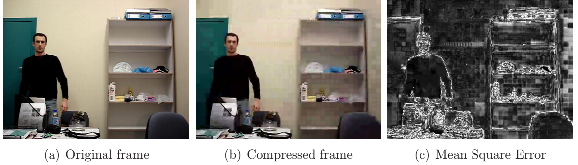
Figure 1.5 Displays of an original video and its compressed version. Some degradations, called artefacts, are present in the compressed video (b). (c) is the error between the original and the compressed video (magnified 5 times for the purpose of display).
