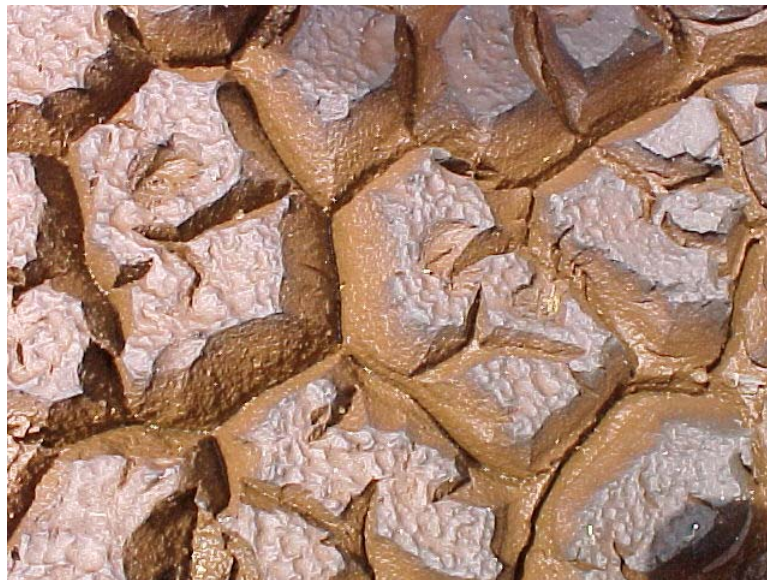
Figure 6.2 Residuals cracked at 10% solids content
