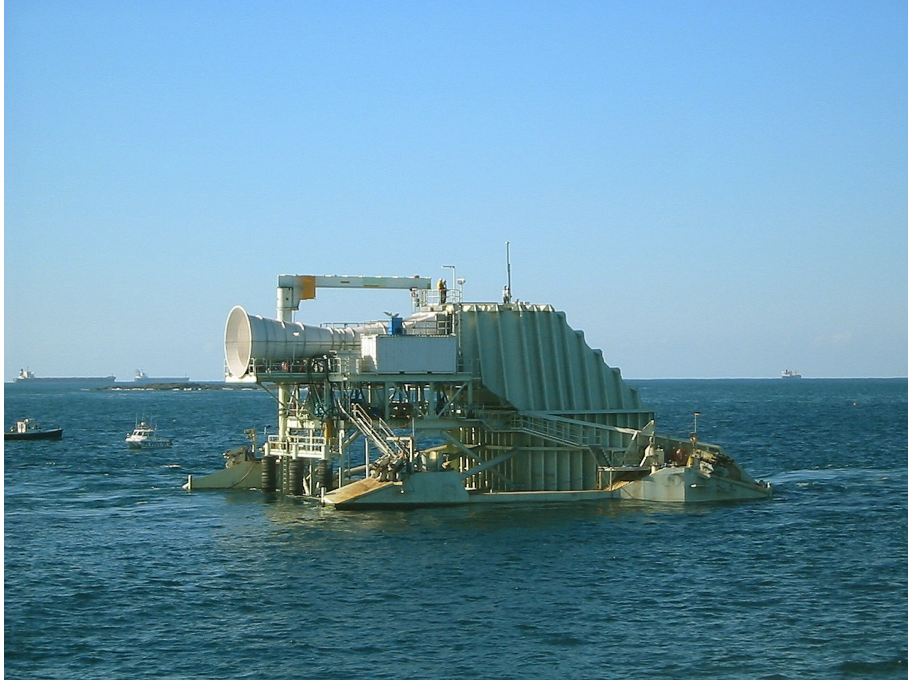
Figure 5.1: An OWC prototype located at Port Kembla, NSW, Australia
