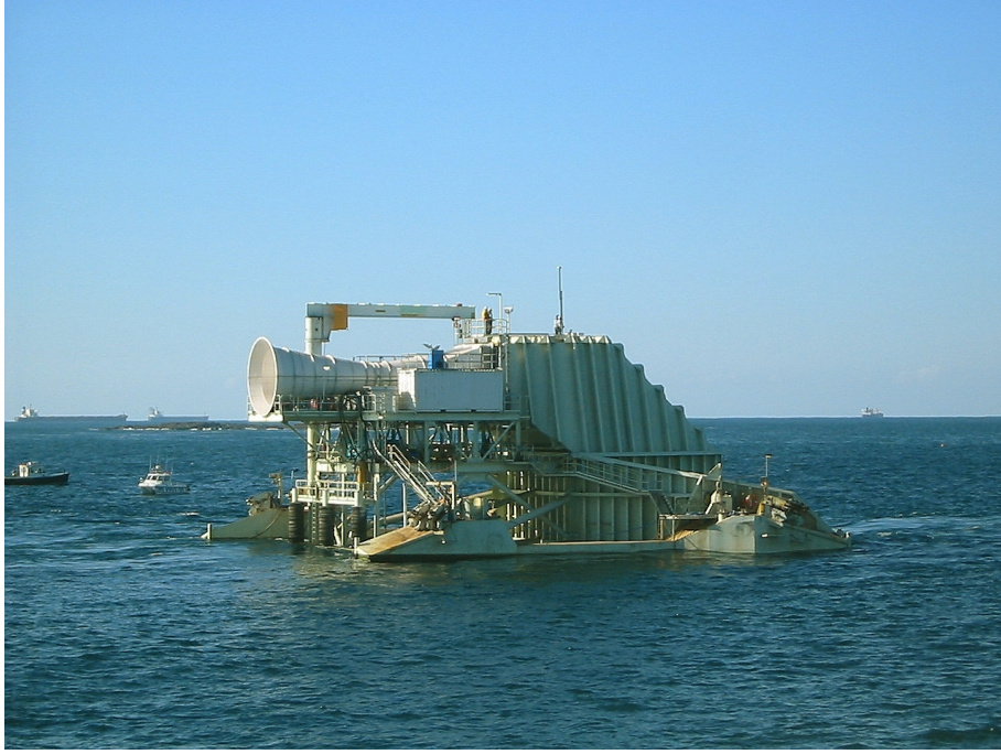
Figure 1.2: An OWC prototype located at Port Kembla, NSW, Australia
