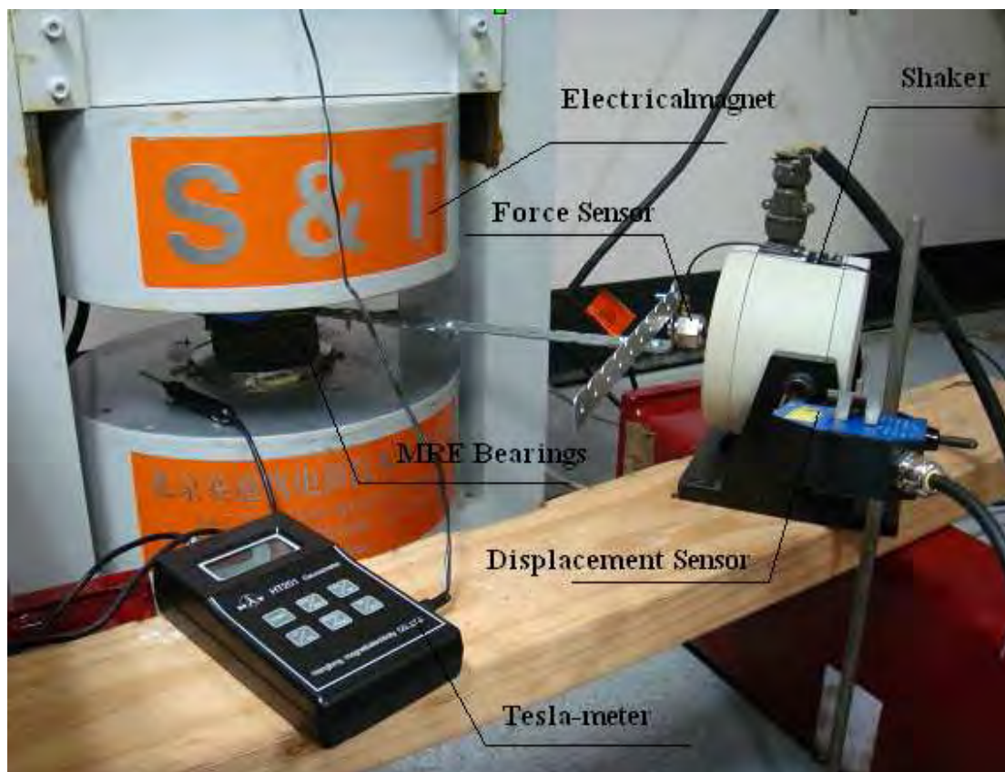
Figure 4.3 Photograph of experiment setup for MRE devices
