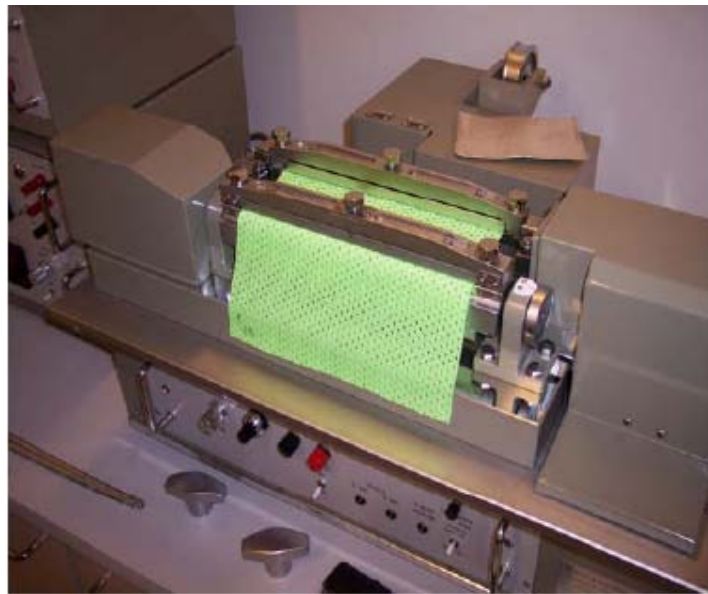
Figure 40. Kawabata Tensile and shear tester
