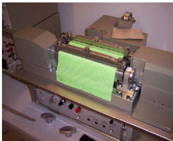
Figure 4. Kawabata Machine- Tensile and Shear tester [5]
