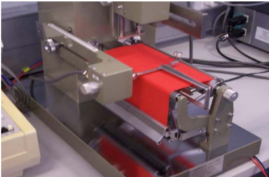
Figure 6. Kawabata Machine-Surface tester [5]
