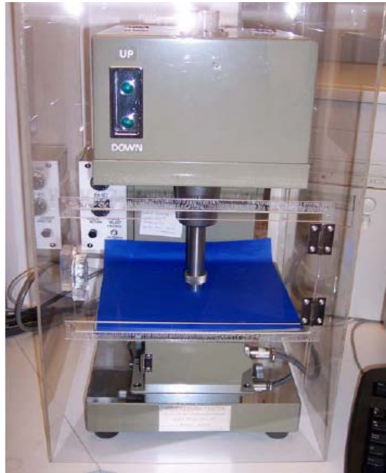
Figure 5. Kawabata Machine- Compression tester [5]
