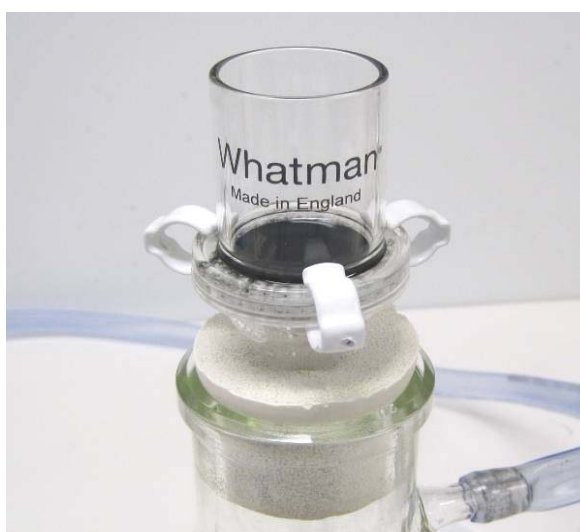
Figure 3.3 Filtration process using Whatman 47 mm filtration cell.
