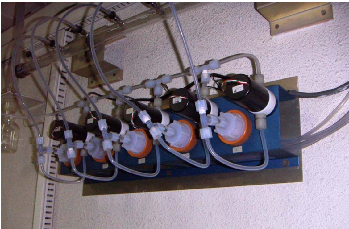
Figure 4.5 Entering filter for gaseous air pollutants
