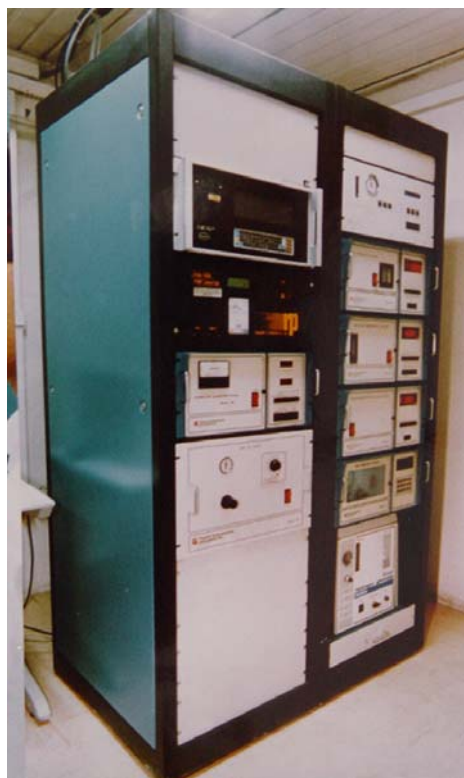
Figure 4.6 Air quality analysers located in AQCC stations
