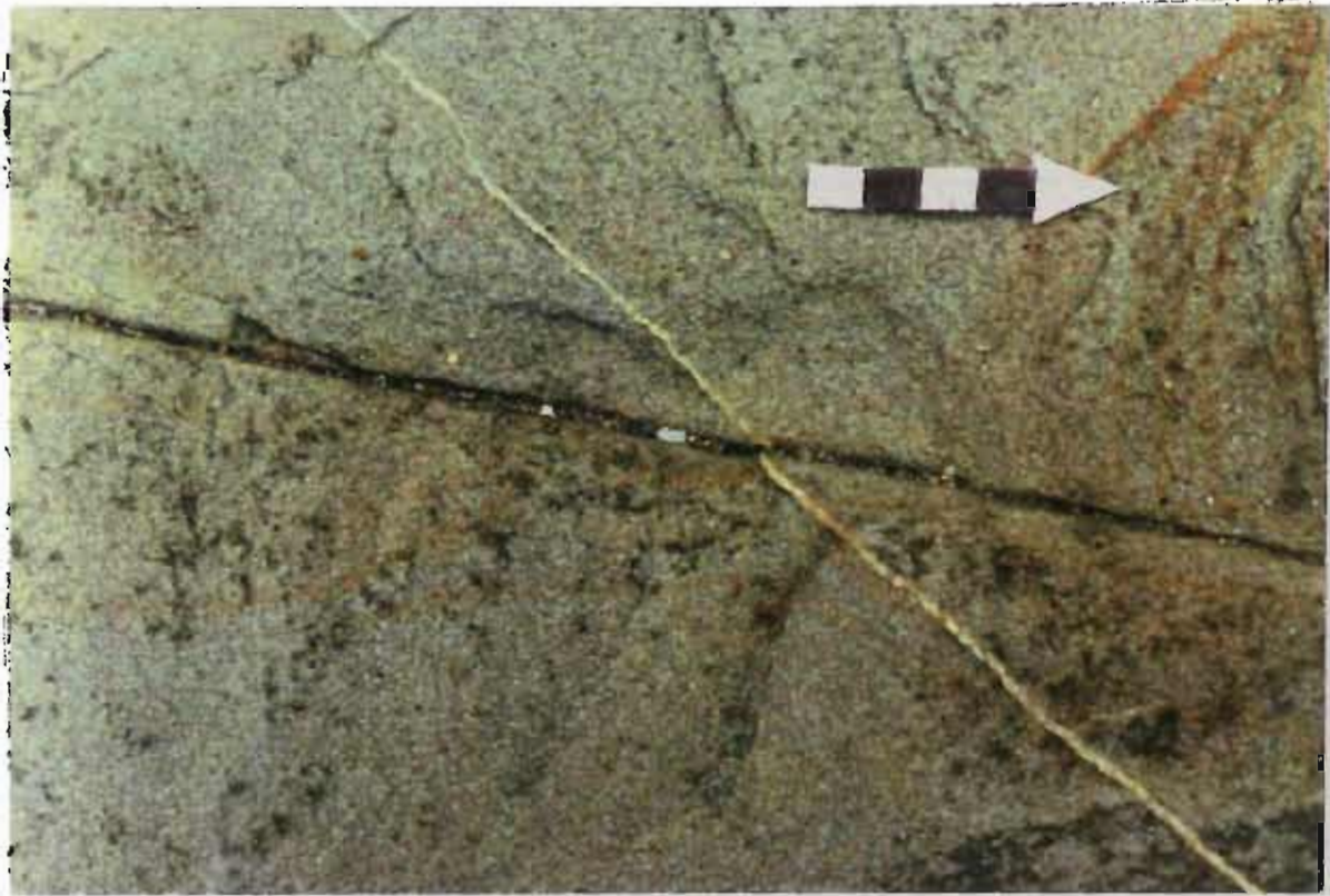
Figure 5.2 A 2 mm dextral movement along a 010^\circ faulted joint which has displaced a 045^\circ joint. The joint infilling is calcite (arrow scale is 5 cm and points to the north).
