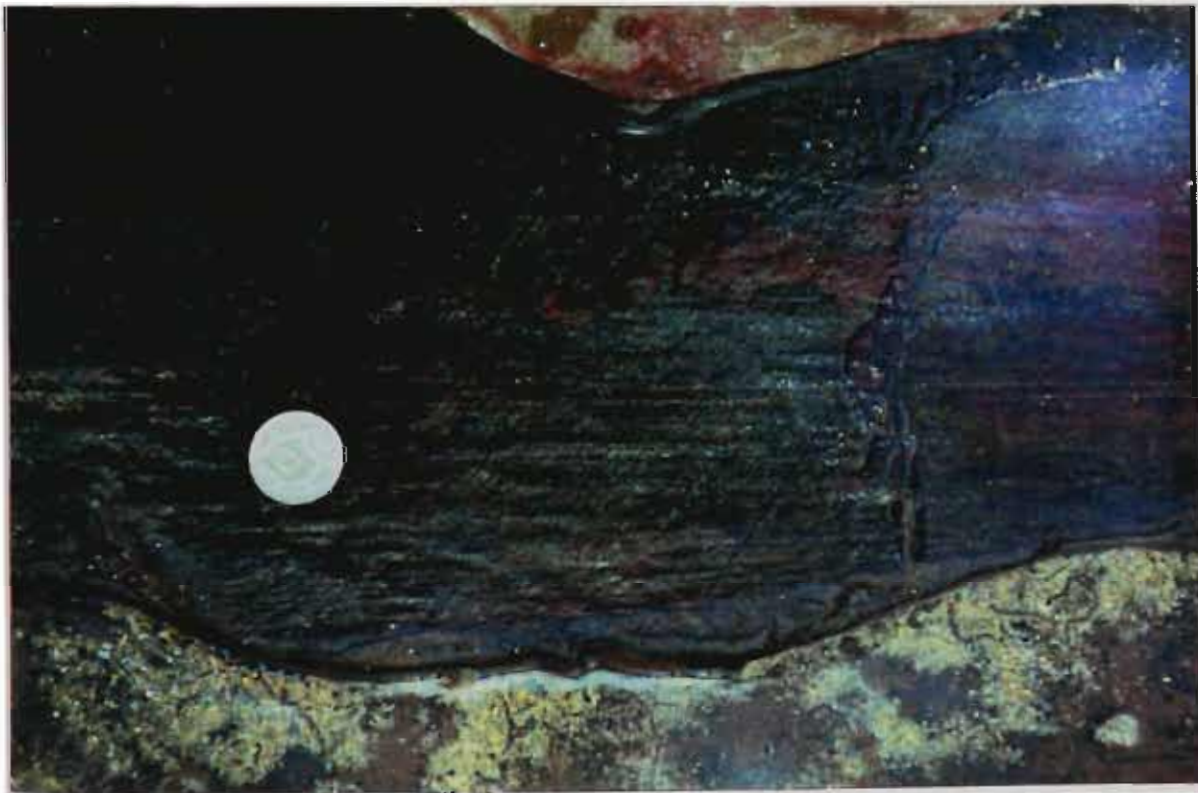
Figure 2.20 Fracture pattern of a silicified plant fragment at Coledale (48 m mark of Scanline 13-AA'). The dominant joint set, strikes 135^\circ with a spacing of 1-2 mm. The second set, which strikes 035-040^\circ , is nonsystematic and abuts against the first set. Coin has 1 cm radius.
