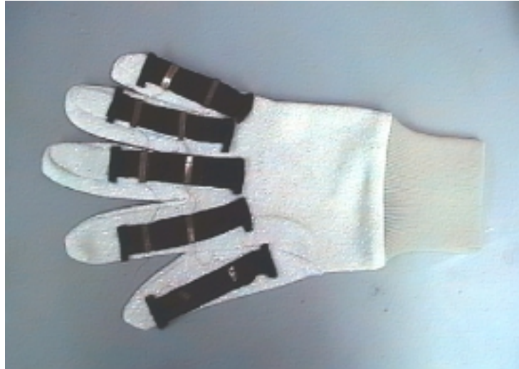
Figure 6.7. The rehabilitation glove with PPy-coated fabric sensor strips on each finger.
