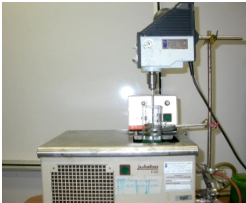
Figure 4.3. Thermobath with temperature control used in the dyeing process.
