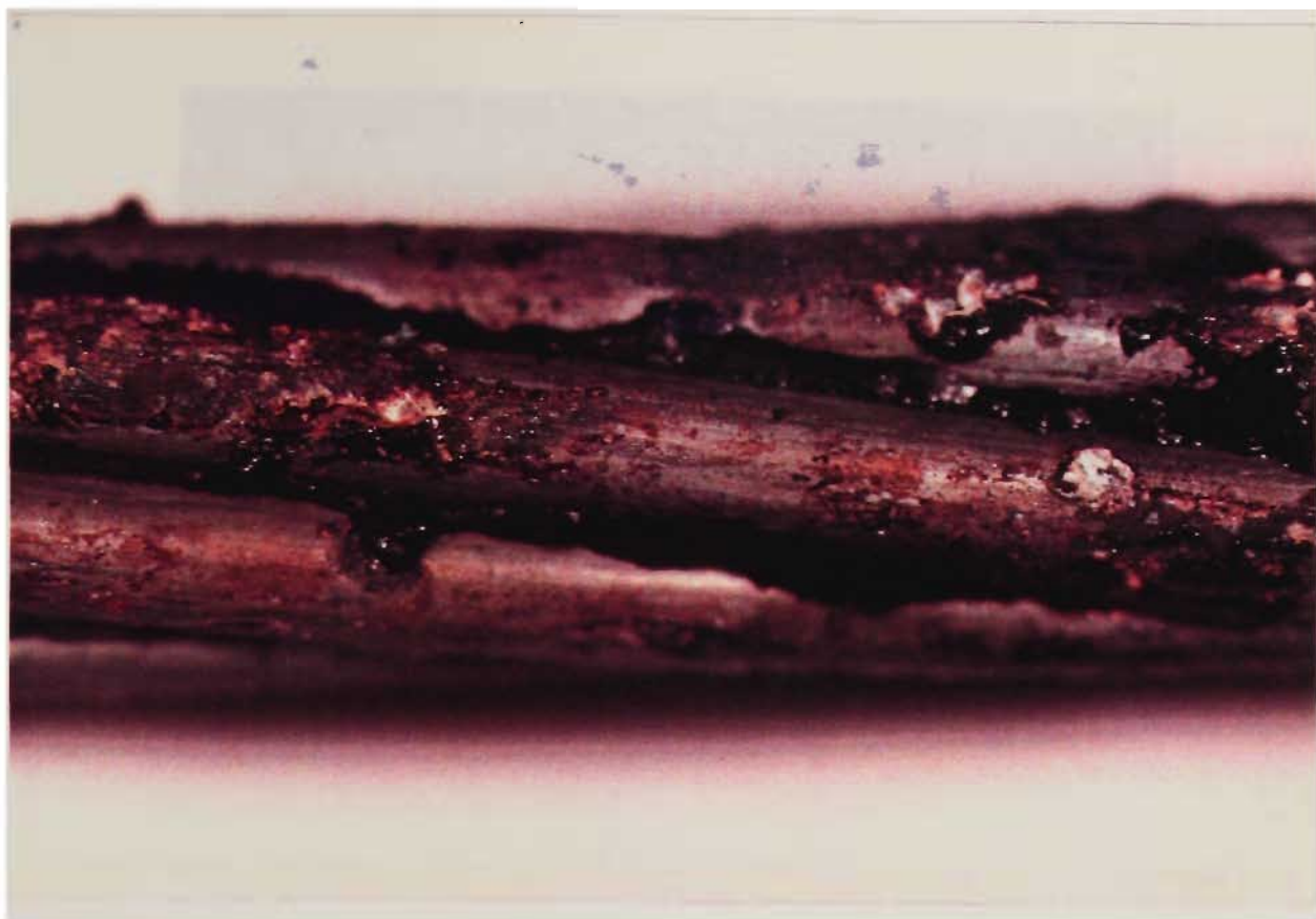
PLATE 3.18 30/7/2.99 MM ACSR/GZ 6 WIRE LAYER AGED AND TARRED SAMPLE AFTER 864 HOURS SALT SPRAY EXPOSURE LOCALISED BROWN STRAINING
