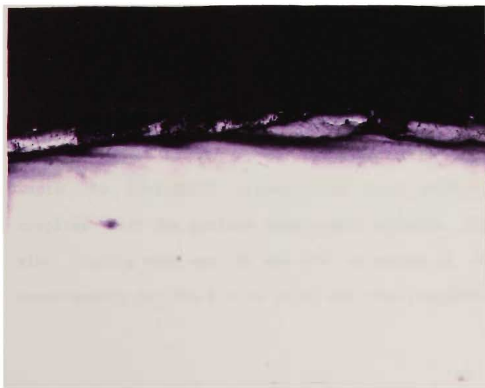
PLATE 3.21 30/7/3.00 MM ACSR/GZ 6 WIRE LAYER NEW AND GREASED SAMPLE AFTER 864 HOURS SALT SPRAY EXPOSURE CROSS SECTION SHOWING LOCALISED LOSS OF ZINC COATING
