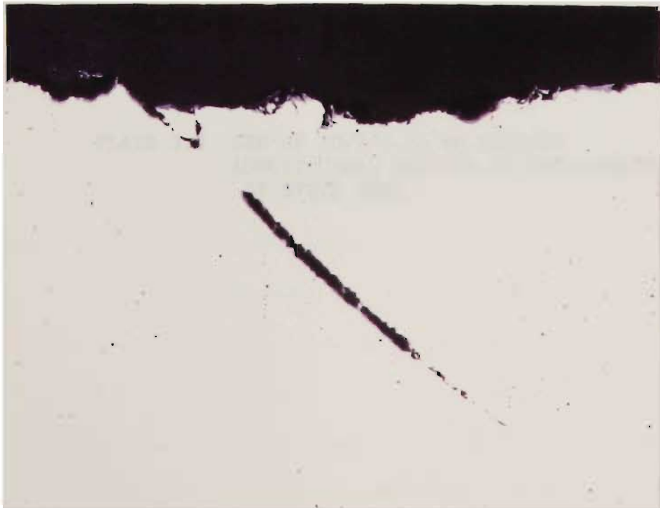
PLATE 3.7 SEM OF 19/3.25 MM AAC LONGITUDINAL SECTION OF FATIGUE CRACK
