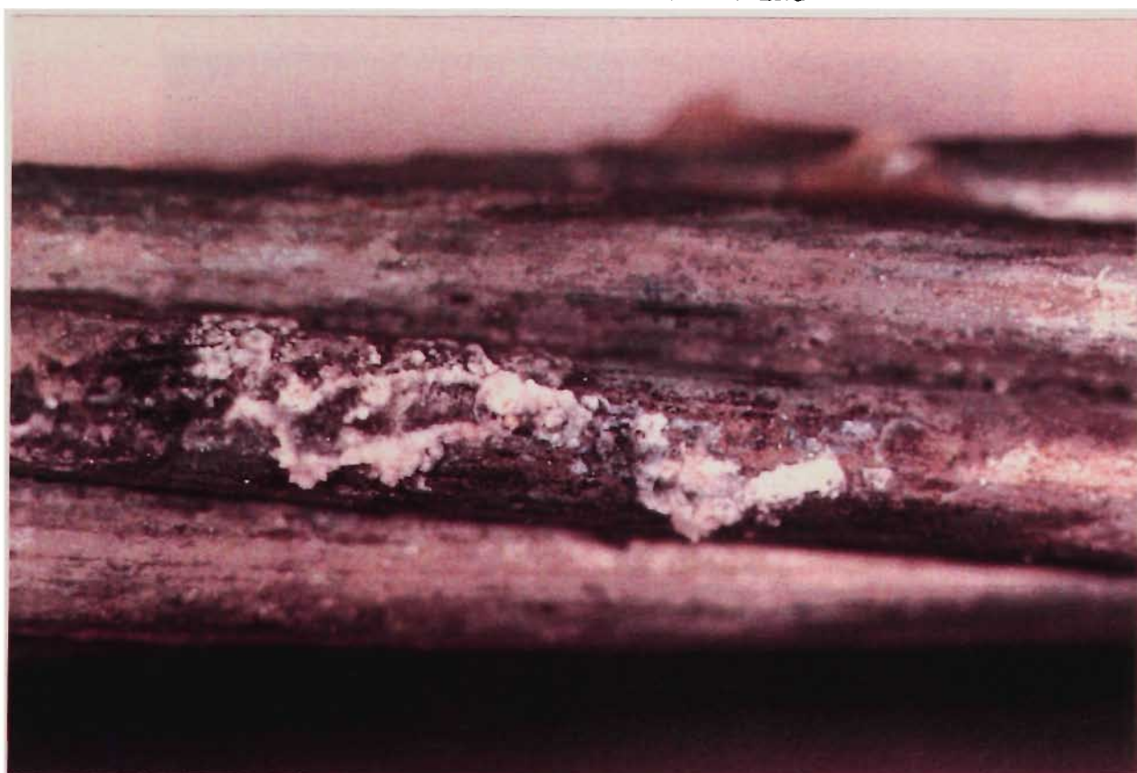
PLATE 3.19 30/7/3.00 MM ACSR/GZ 6 WIRE LAYER NEW AND GREASED SAMPLE AFTER 864 HOURS SALT SPRAY EXPOSURE LOCALIZED DISCOLOURATION OF ZINC COATING
