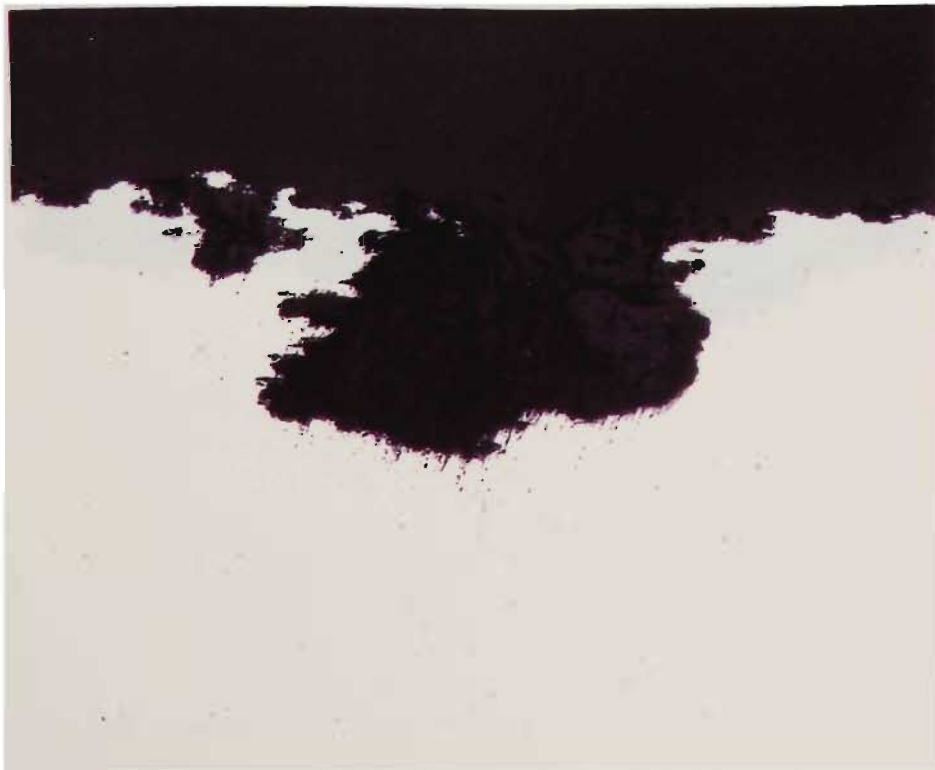
PLATE A3.25 - LONGITUDINAL SECTION OF 18 WIRE LAYER ALUMINIUM PITTING FROM TOMAGO TO TAREE TRANSMISSION LINE X50
