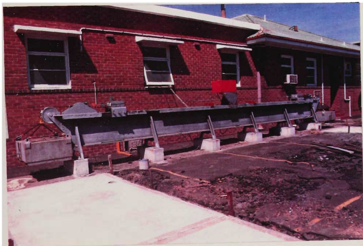
PLATE 4.3 GENERAL ARRANGEMENT OF CONDUCTOR FATIGUE TESTER
