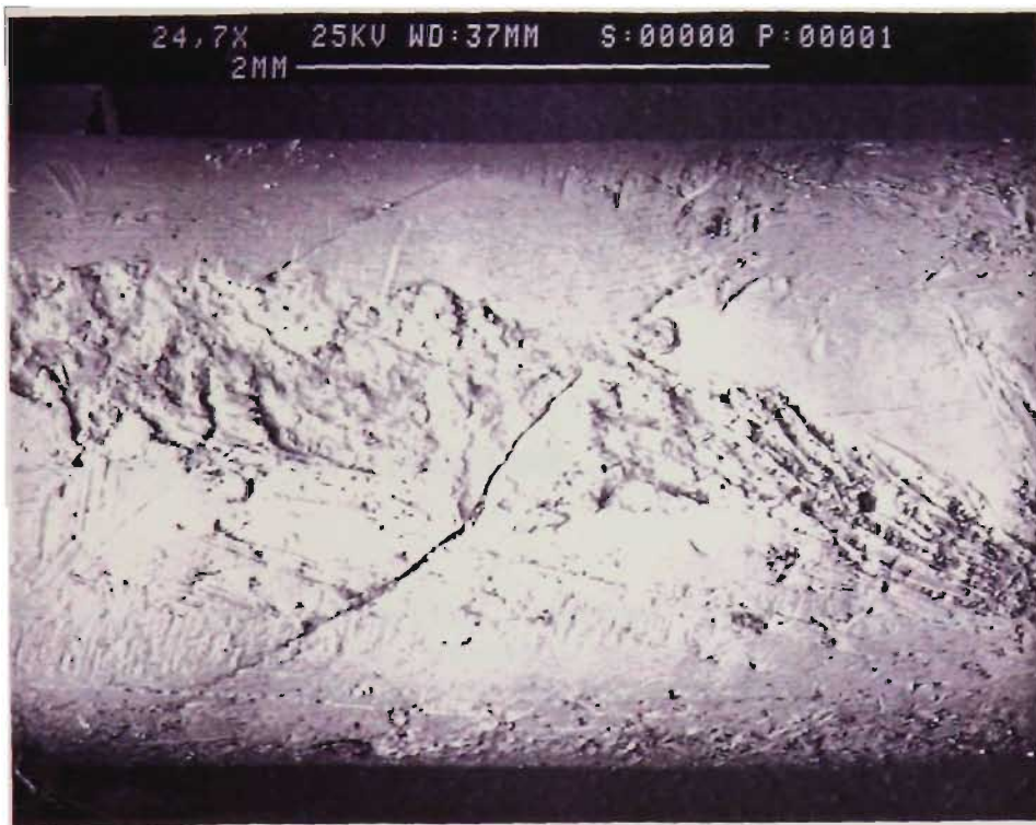
PLATE 3.3 19/3.25 AAC CONDUCTOR CONDUCTOR FRETTING AND FATIGUE CRACK
