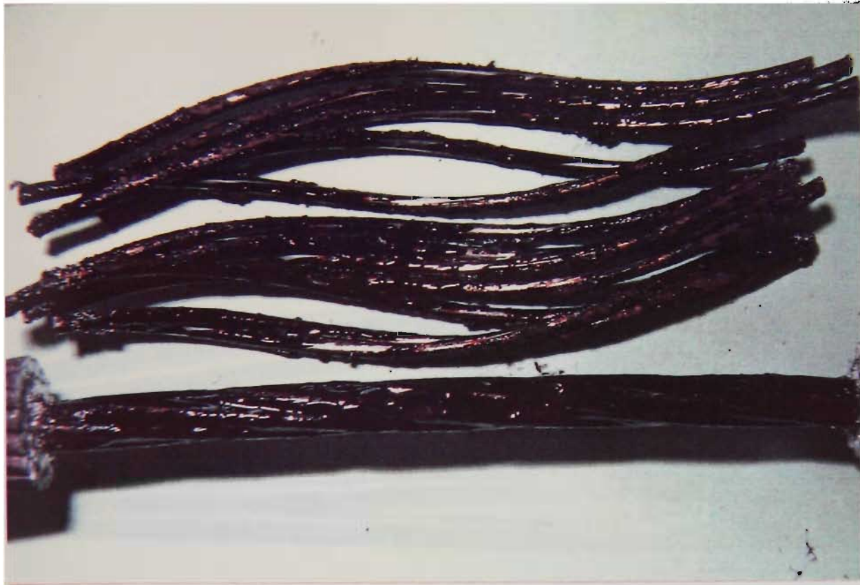
PLATE A3.19 - BELLAMBI TO HEATHCOTE TRANSMISSION LINE 6 WIRE STEEL LAYER AND UNDERSIDE OF THE 12 WIRE ALUMINIUM LAYER
