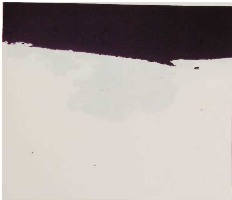
PLATE A3.23 - LONGITUDINAL SECTION OF ELLIPTICAL AREA DAMAGE OF ALUMINIUM STRANDS X100
