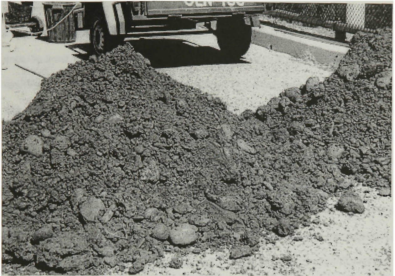
Figure 7.13 Sandy gravel 'transition zone' material from an embankment dam
