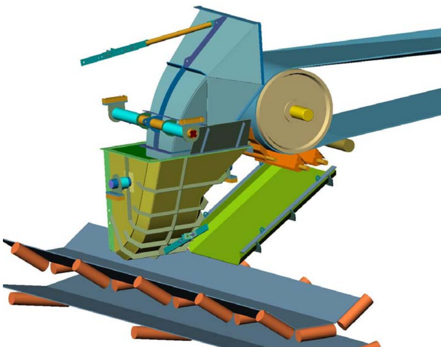
Figure 7.2 Image depicting hood-spoon transfer chute system – view two
