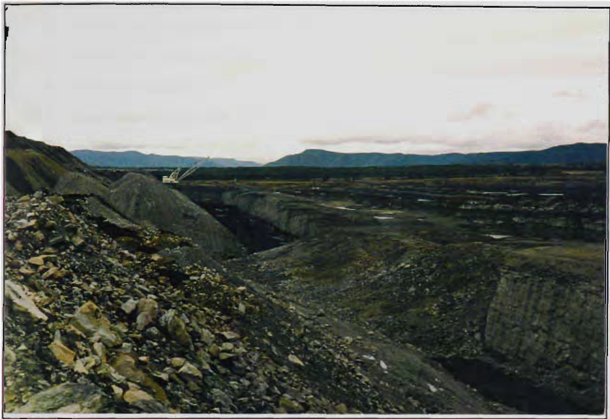
Figure 2.12- An example of the throw blasting technique used for a dragline pit.
