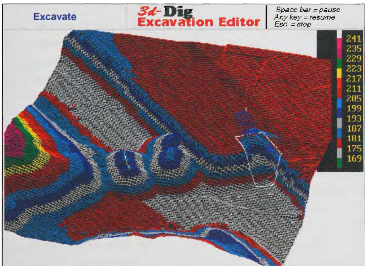
Figure 3.10 - A 3D view of a simulated pit created by 3D DIG software.
