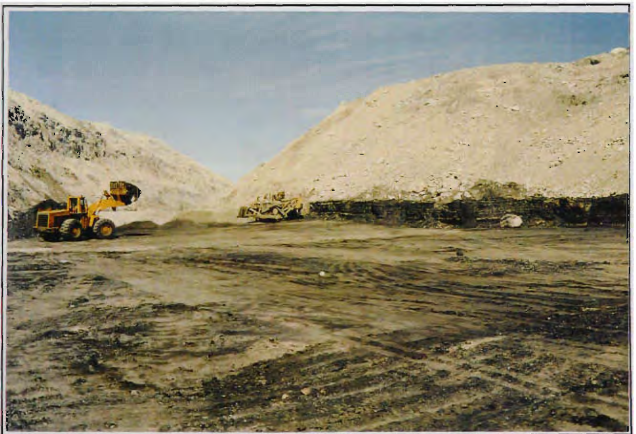
Figure 10.17- The use of loader and dozers as support equipment for coal loading and haulage operation at the case study mine.
