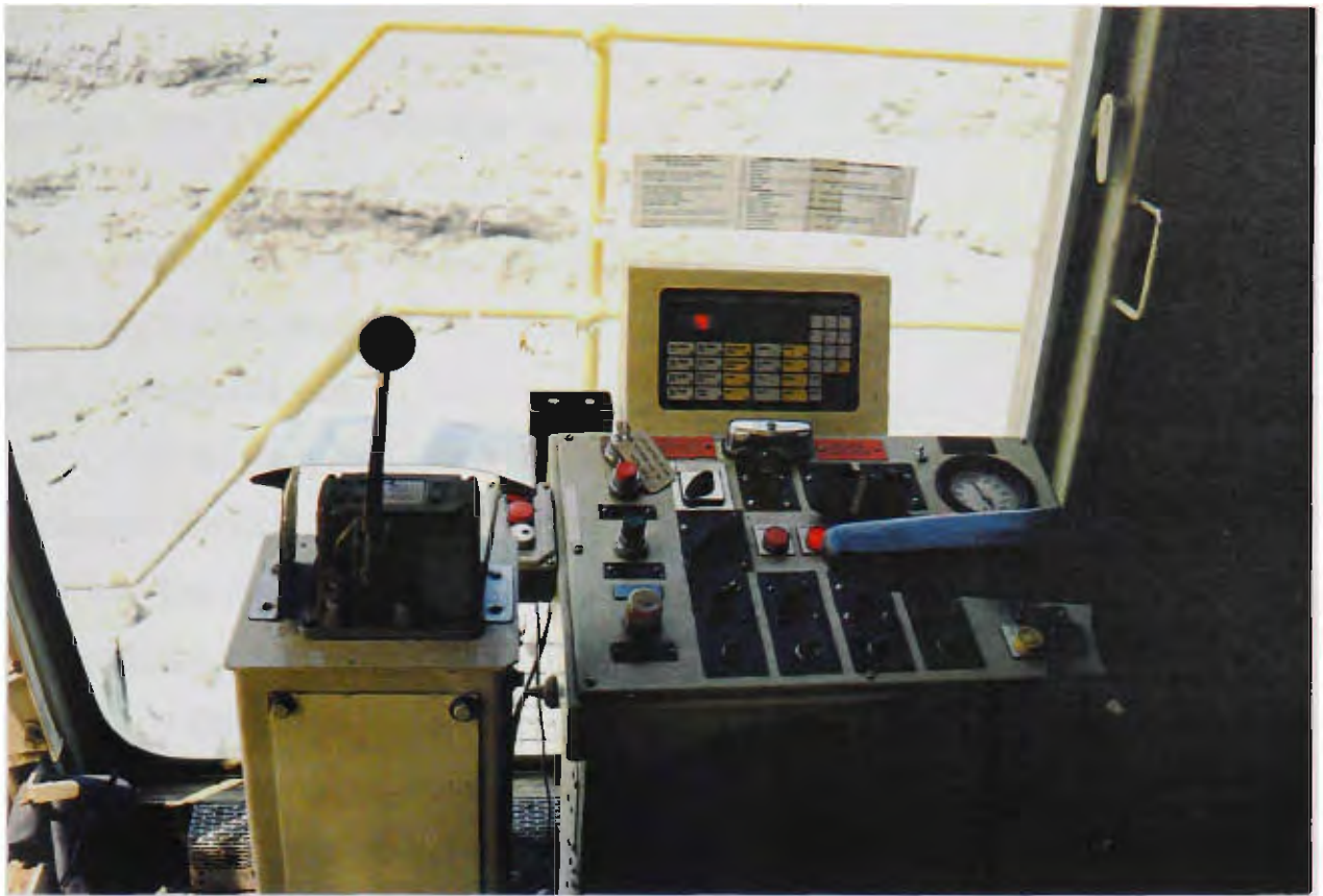
Figure 7.2- On-board equipment of a Tritronics 9000 dragline monitoring system.
