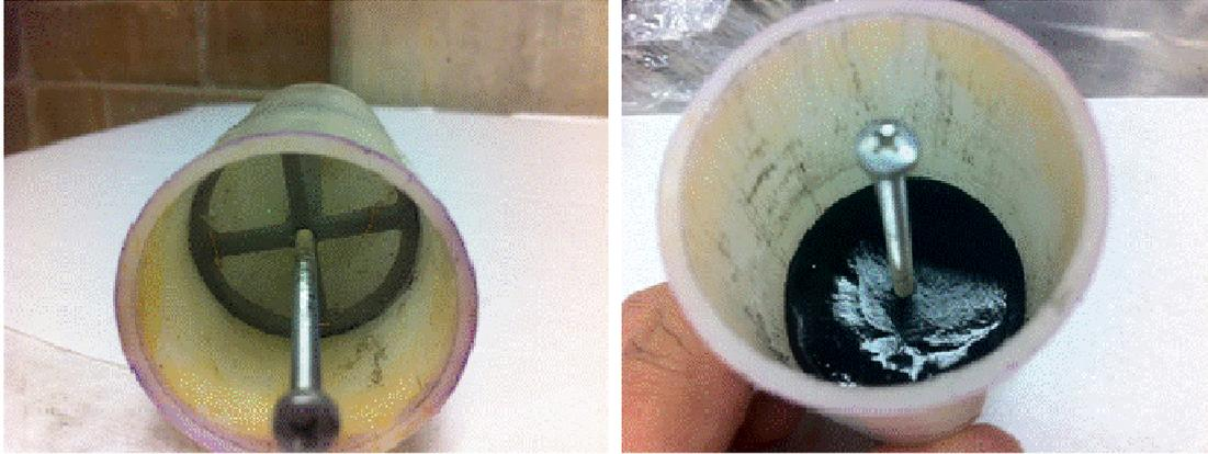
Fig. 1. Modified centrifuge tube before and after test. The photo on the left shows the dewatered cake formed above the centrate in the modified centrifugal test
