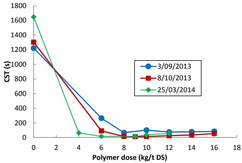
Fig. 3. OPD<sub>CST</sub> on different sampling days
