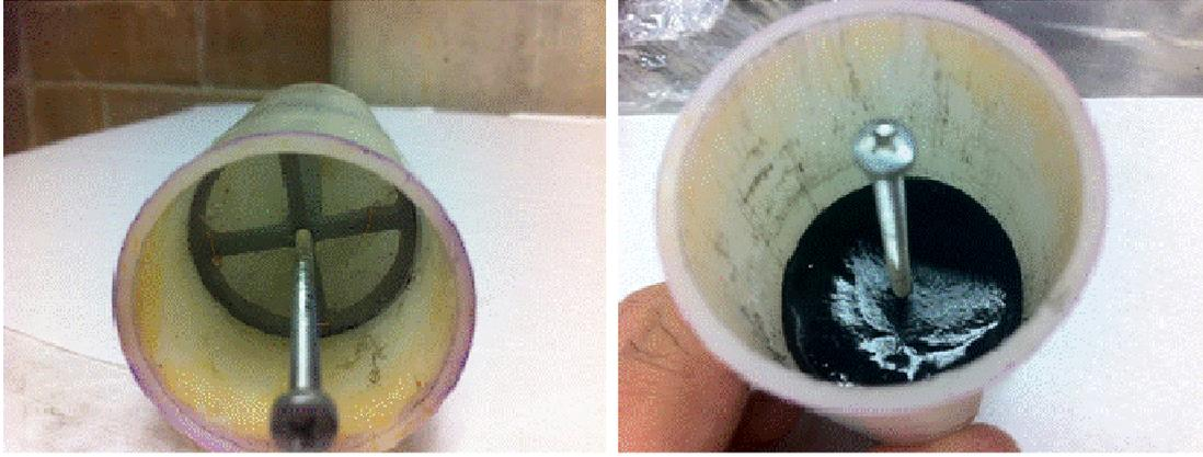
Fig. 1. Modified centrifuge tube before and after test. The photo on the left shows the dewatered cake formed above the centrates in the modified centrifugal test
