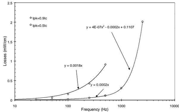
Figure 12. Frequency dependence of ac loss of P.1.
