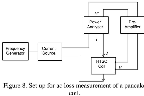
Figure 8. Set up for ac loss measurement of a pancake coil.
