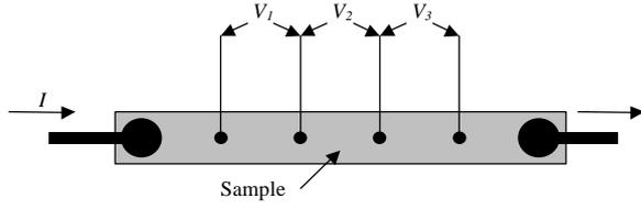
Figure 2. Configuration of sample for I-V measurements.
