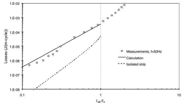
Figure 10. Losses in P.1 carrying ac transport current.
