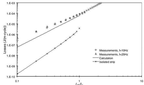
Figure 11. Losses in P.2 carrying ac transport current.
