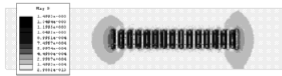
Figure 13. A magnetic field map of a non-inductive coil.
