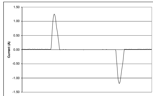
Fig. 12. 17 inch LCD Monitor Input Current Waveform
