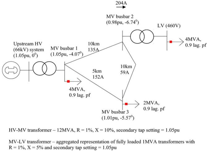
Fig. 7. Three-bus MV test system.
