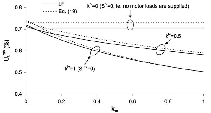
Fig. 4. Variation of  $U_t^{mv}$  with  $k_m$  for cases where  $k^{lv} = 1$ ,  $k^{lv} = 0.5$ , and  $k^{lv} = 0$ .
