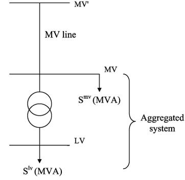
Fig. 2. MV-LV radial system.
