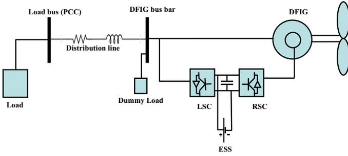
Fig. 1. DFIG based RAPS system with ESS unit
