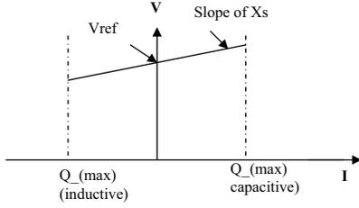
Fig. 3. Wind turbine V-I characteristics
