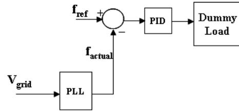
Fig. 4. Dummy load controller
