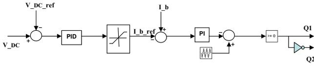
Fig. 5. Control strategy for the battery storage system
