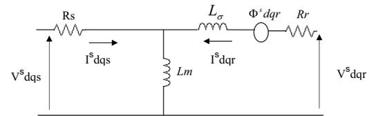
Fig. 2. ISFO equivalent circuit of a DFIG
